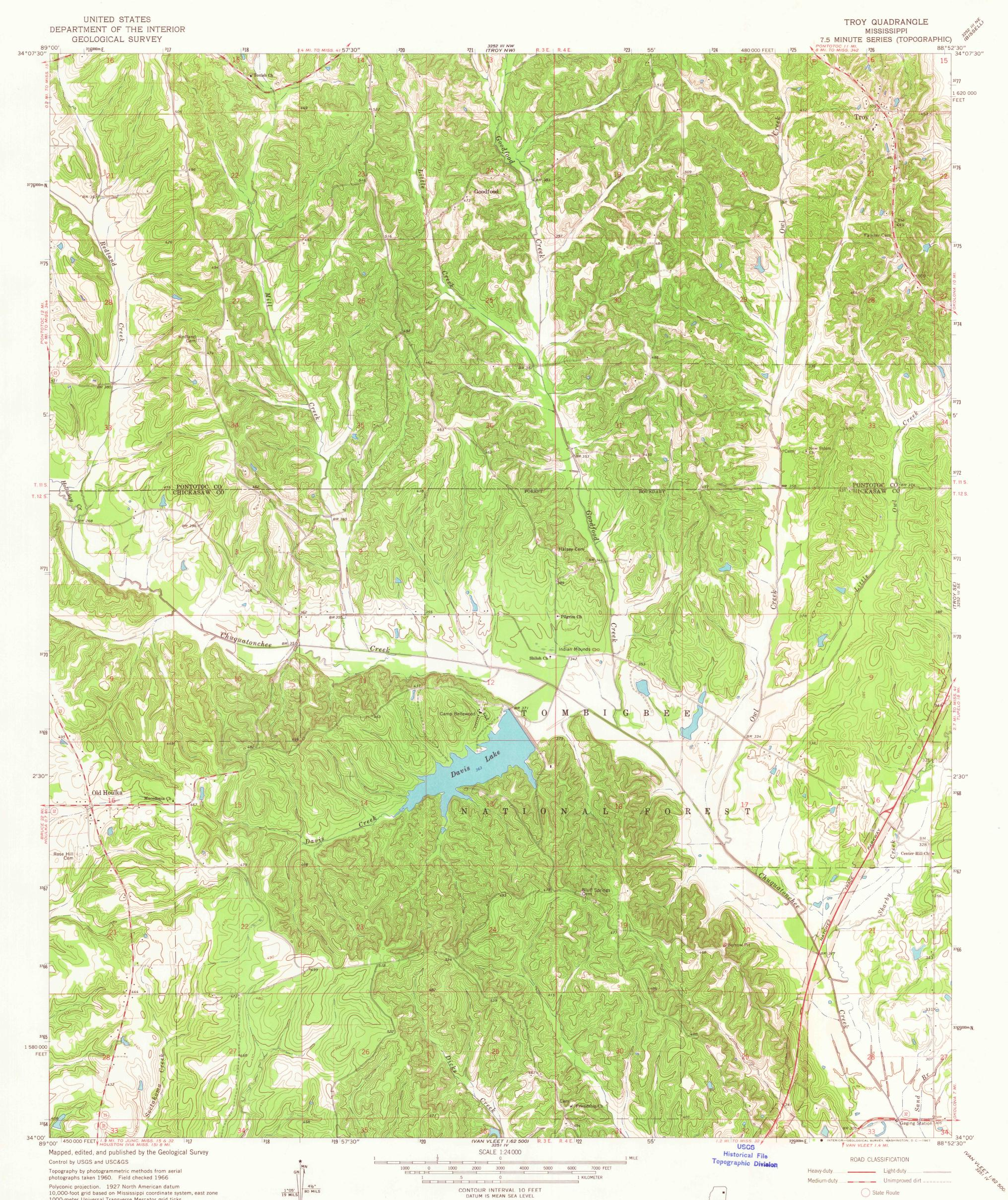
10,000-foot grid based on Mississippi coordinate system, east zone 1000-meter Universal Transverse Mercator grid ticks, zone 16, shown in blue
