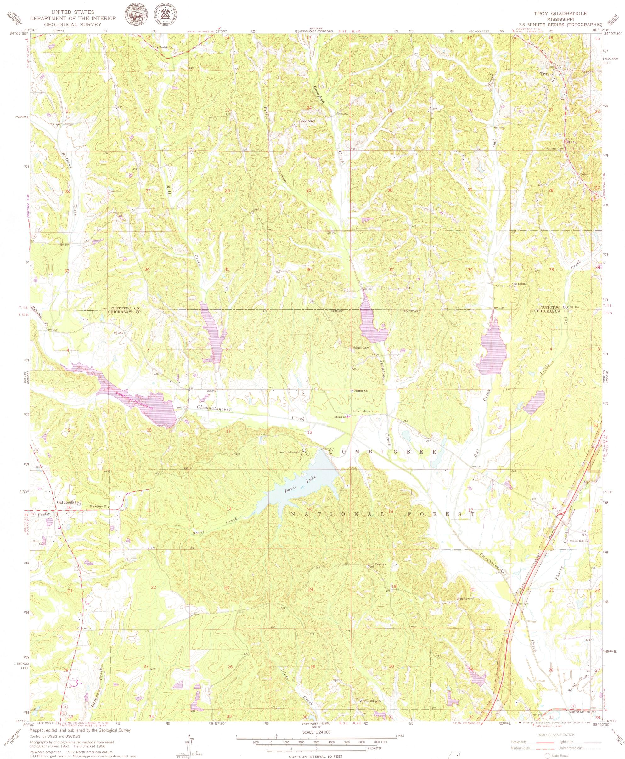
10,000-foot grid based on Mississippi coordinate system, east zone To place on the predicted North American Datum 1983 move the projection lines 9 meters south and 5 meters east as shown by dashed corner ticks 1000-meter Universal Transverse Mercator grid ticks, zone 16, shown in blue
