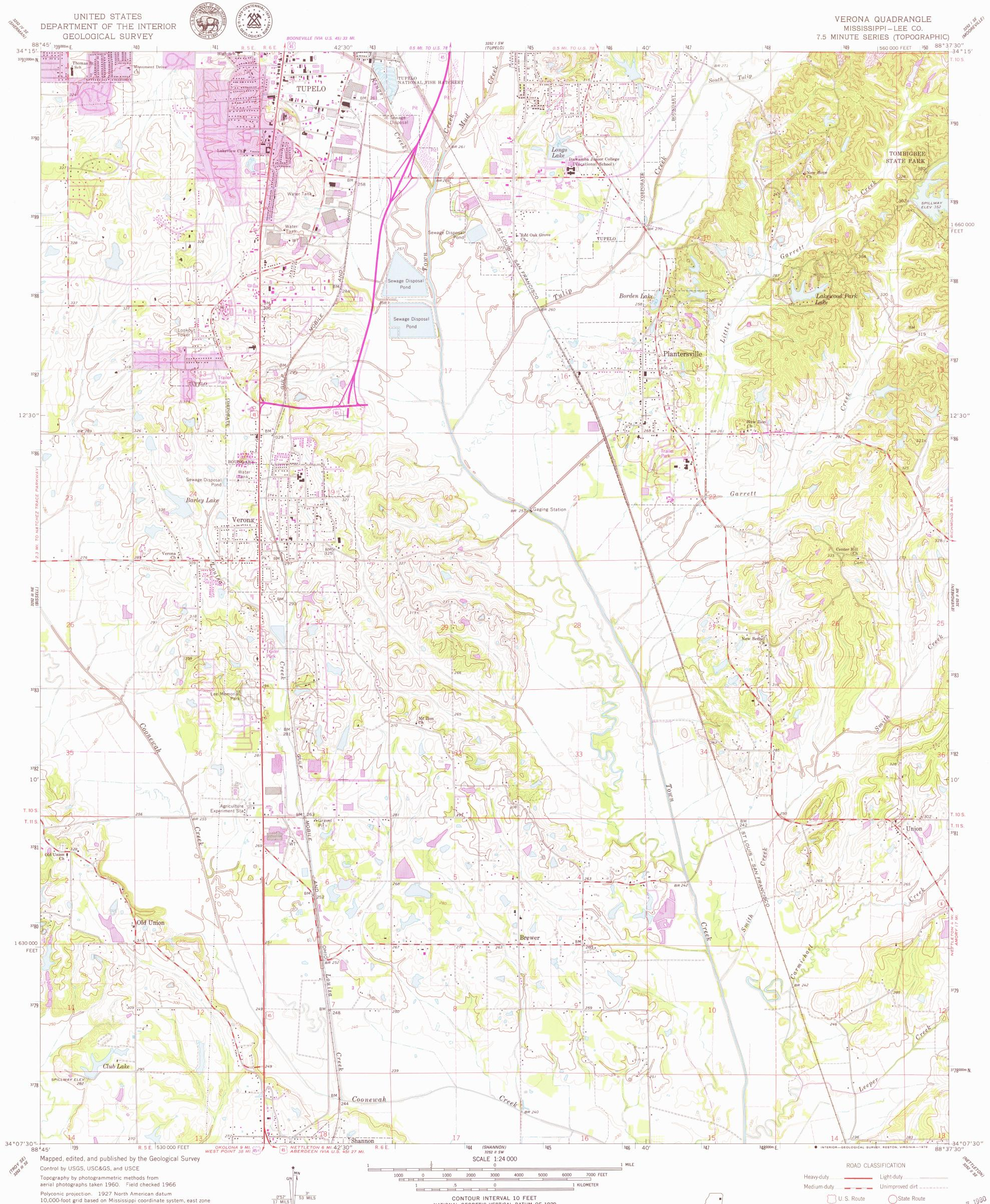
10,000-foot grid based on Mississippi coordinate system, east zone To place on the predicted North American Datum 1983 move the projection lines 9 meters south and 4 meters east as shown by dashed corner ticks 1000-meter Universal Transverse Mercator grid ticks, zone 16, shown in blue
