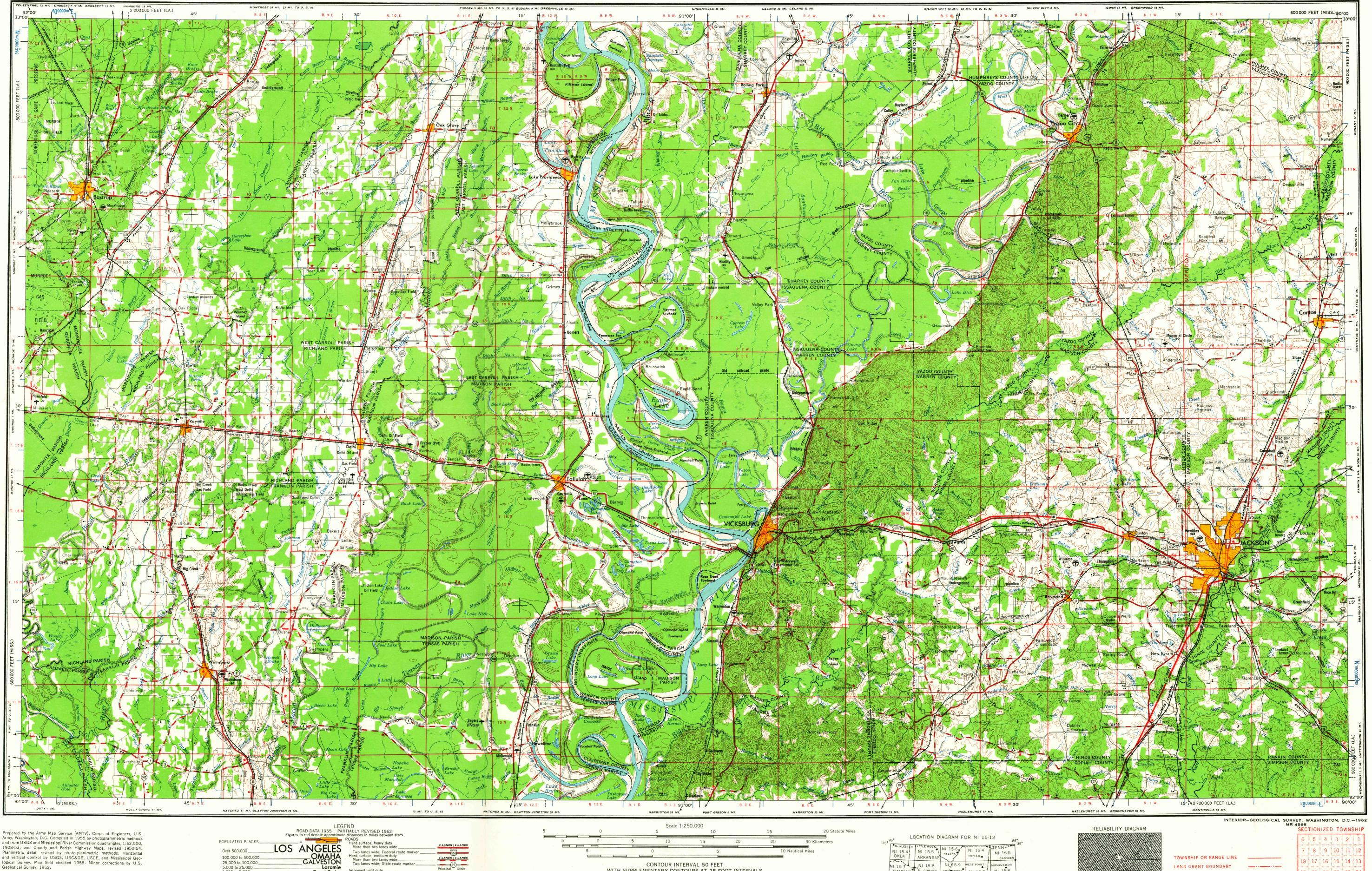
Prepared by the Army Map Service (AMTV), Corps of Engineers, U.S. Army, Washington, D.C. Compiled in 1955 by photogrammetric methods and from USGS and Mississippi River Commission quadrangles, 1:62,500, 1908-53; and County and Parish Highway Maps, revised 1950-54. Planimetric detail revised by photo-planimetric methods. Horizontal and vertical control by USGS, USC&GS, USCE, and Mississippi Geological Survey. Map field checked 1955. Minor corrections by U.S. Geological Survey, 1962.
