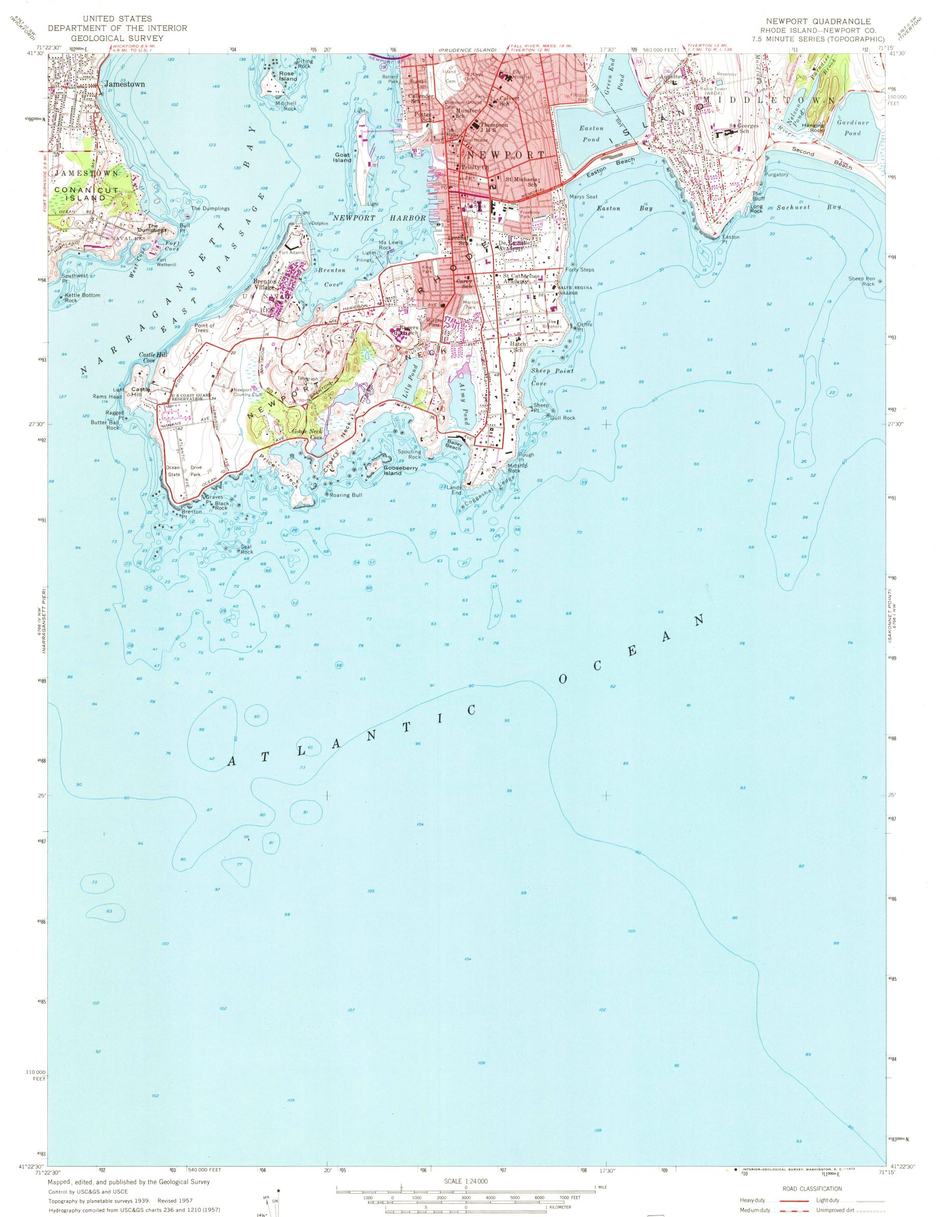
Polyconic projection. 1927 North American datum 10,000-foot grid based on Rhode Island coordinate system, 1000-meter Universal Transverse Mercator grid ticks, zone 19, shown in blue
