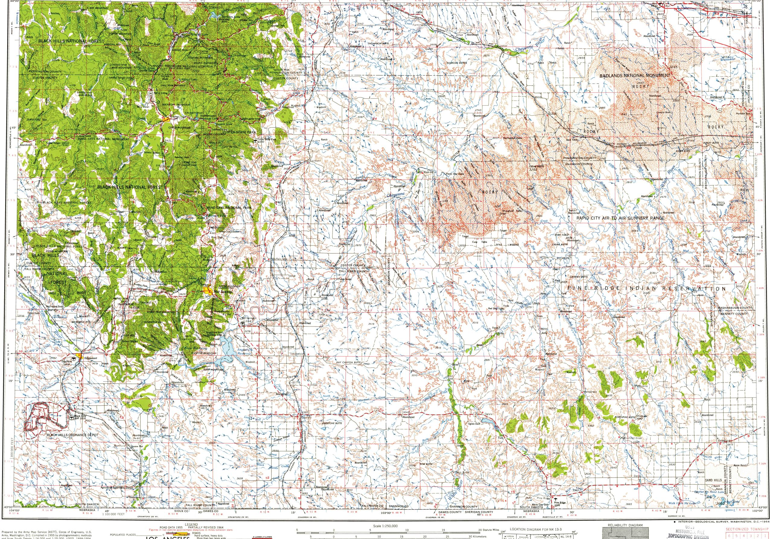
Prepared by the Army Map Service (ASTT), Corps of Engineers, U.S. Army, Washington, D.C. Compiled in 1955 by photogrammetric methods and from South Dakota 1:24,000 and 1:25,000, USGS, 1898-1954. Planimetric detail revised by photo-planimetric methods. Horizontal and vertical control by USGS, USC&GS and USCE. Photography field annotated 1955. Limited revision by U.S. Geological Survey 1964
