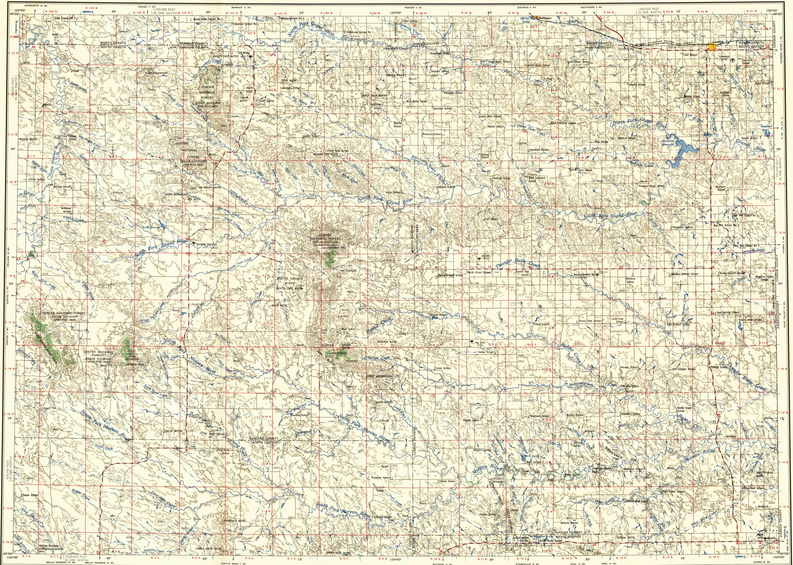
Prepared by the Army Map Service (ASX), Corps of Engineers, U. S. Army, Washington, D. C. Compiled in 1955 by photogrammetric methods and from South Dakota, 1:24,000, USGS, 1951-52. Planimetric detail revised by photogrammetric methods. Horizontal and vertical control by USCGS, USGS and CE. Photography field annotated 1954.
