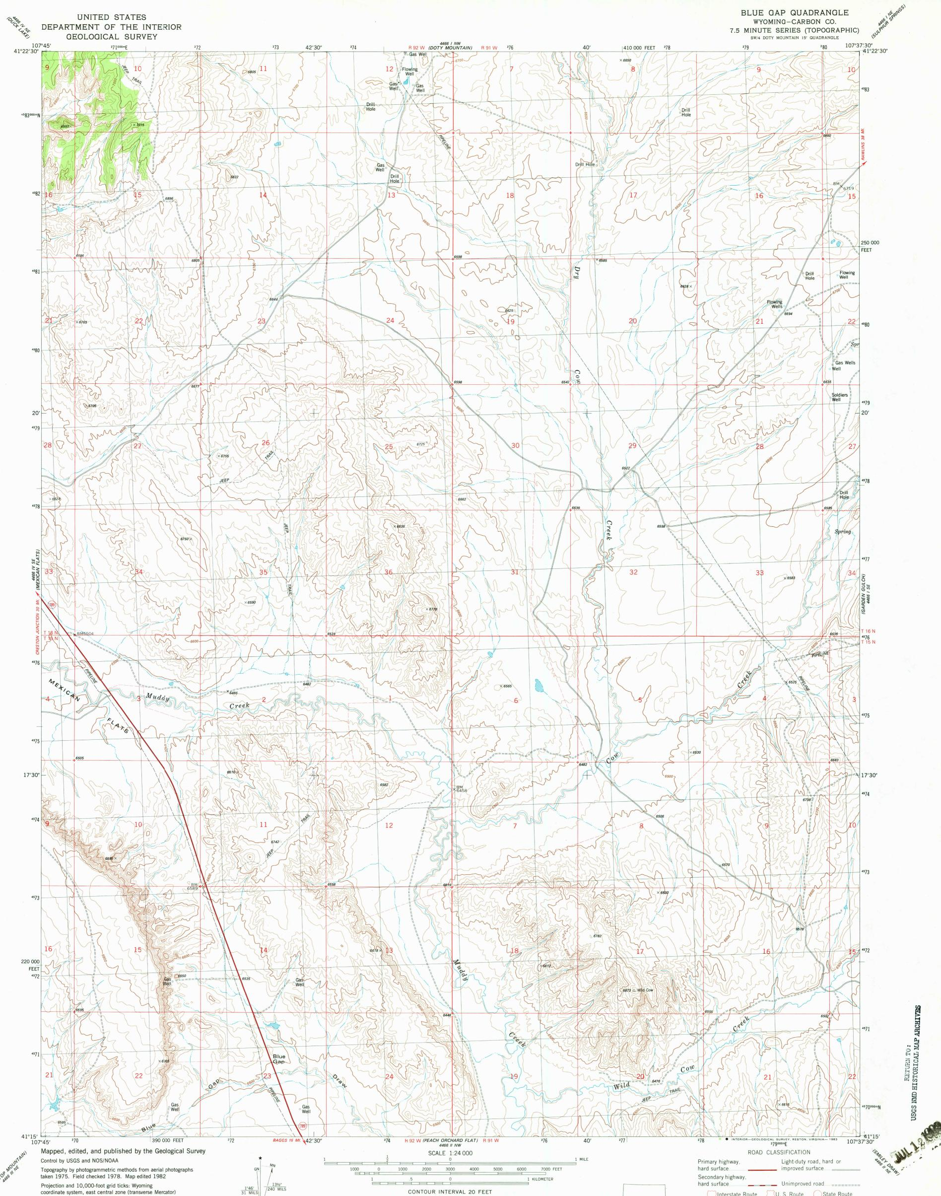
Projection and 10,000-foot grid ticks: Wyoming coordinate system, east central zone (transverse Mercator) 1000-meter Universal Transverse Mercator grid, zone 13 1927 North American datum To place on the predicted North American Datum 1983 move the projection lines 7 meters north and 53 meters east as shown by dashed corner ticks Fine red dashed lines indicate selected fence lines
