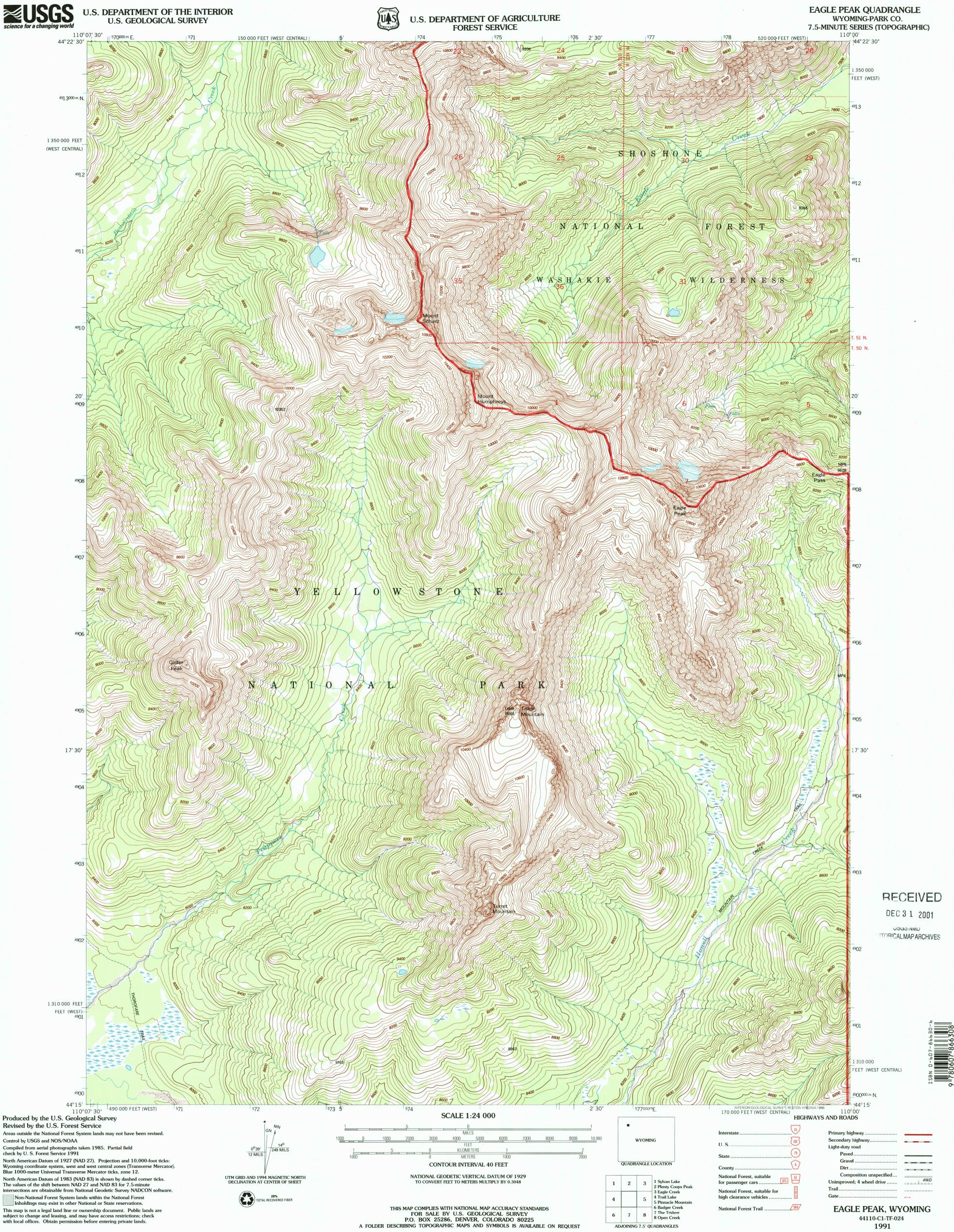
Wyoming coordinate system, west and west central zones (Transverse Mercator). Blue 1000-meter Universal Transverse Mercator ticks, zone 12. North American Datum of 1983 (NAD 83) is shown by dashed corner ticks. The values of the shift between NAD 27 and NAD 83 for 7.5-minute intersections are obtainable from National Geodetic Survey NADCON software.
