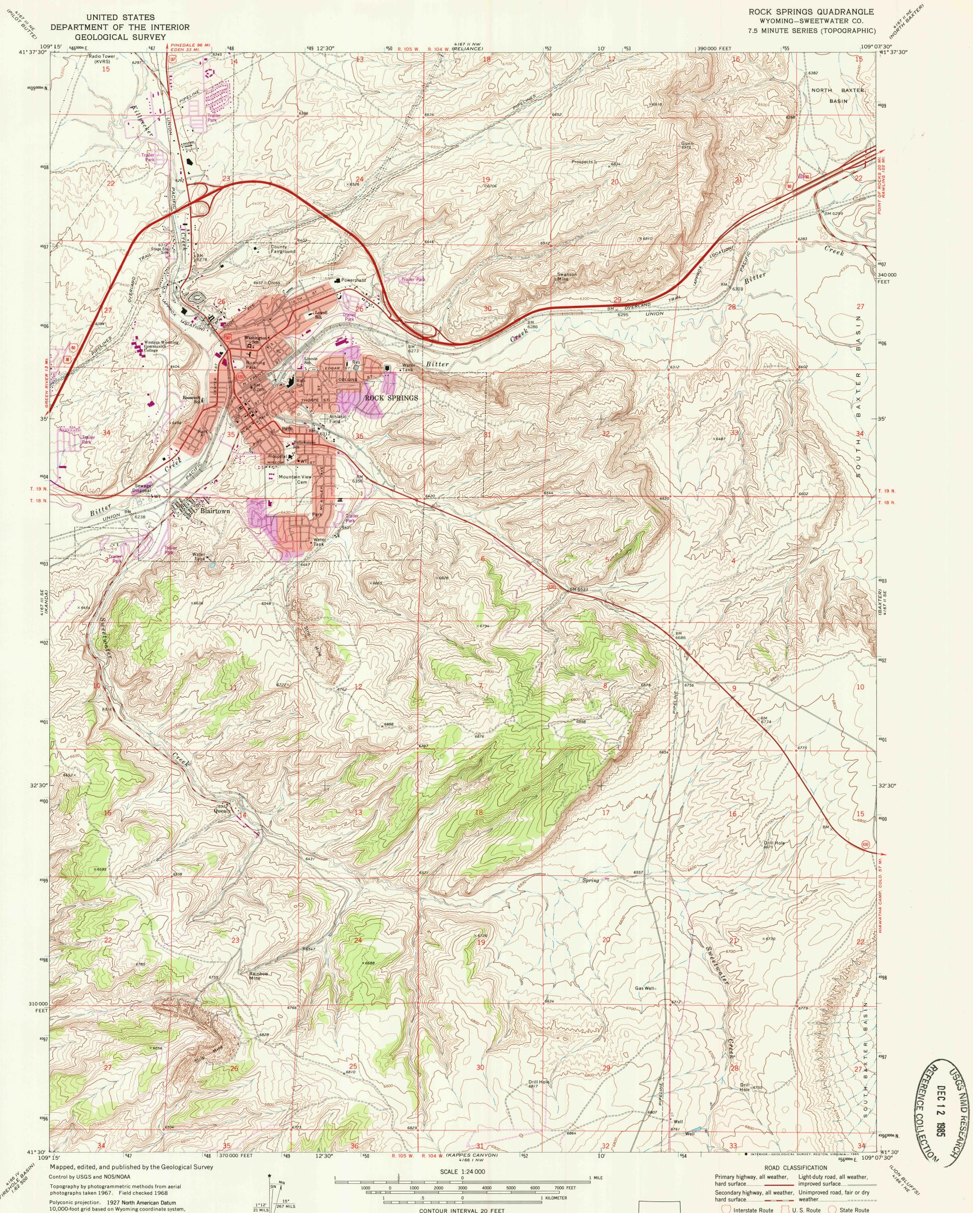
10,000-foot grid based on Wyoming coordinate system, west central zone 1000-meter Universal Transverse Mercator grid ticks, zone 12, shown in blue
