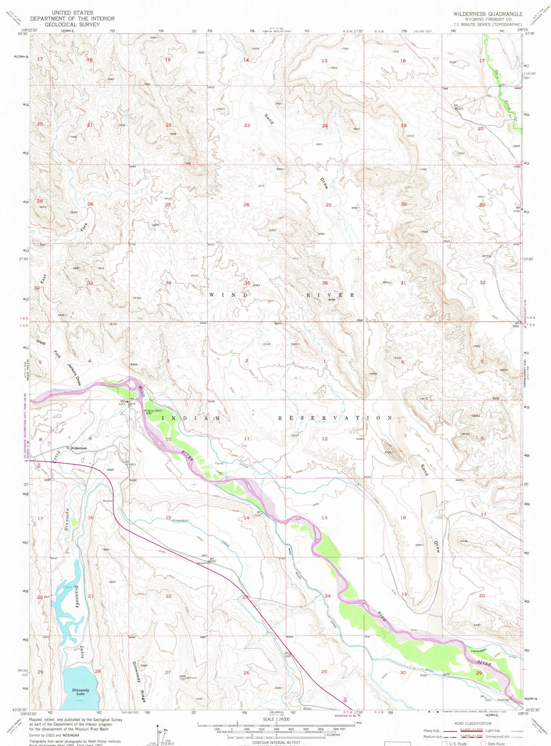
Topography from aerial photographs by Kelsh Plotter methods Aerial photographs taken 1949. Field check 1952 Polyconic projection. 1927 North American datum 10,000-foot grid based on Wyoming coordinate system, west central zone 1000-meter Universal Transverse Mercator grid ticks, zone 12, shown in blue
