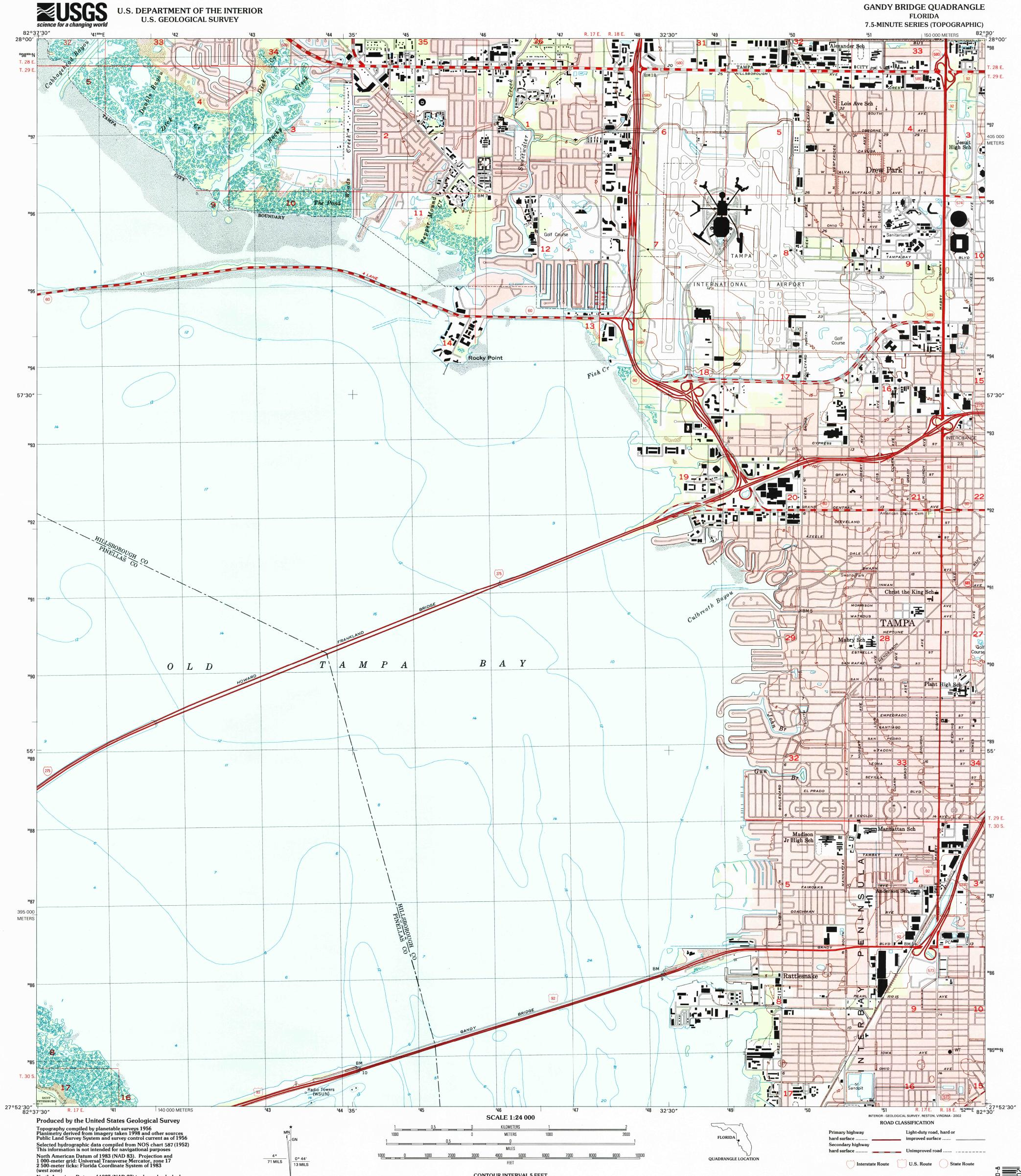
North American Datum of 1927 (NAD 27) is shown by dashed corner ticks. The values of the shift between NAD 83 and NAD 27 for 7.5-minute intersections are obtainable from National Geodetic Survey NADCON software Landmark buildings verified 1956
