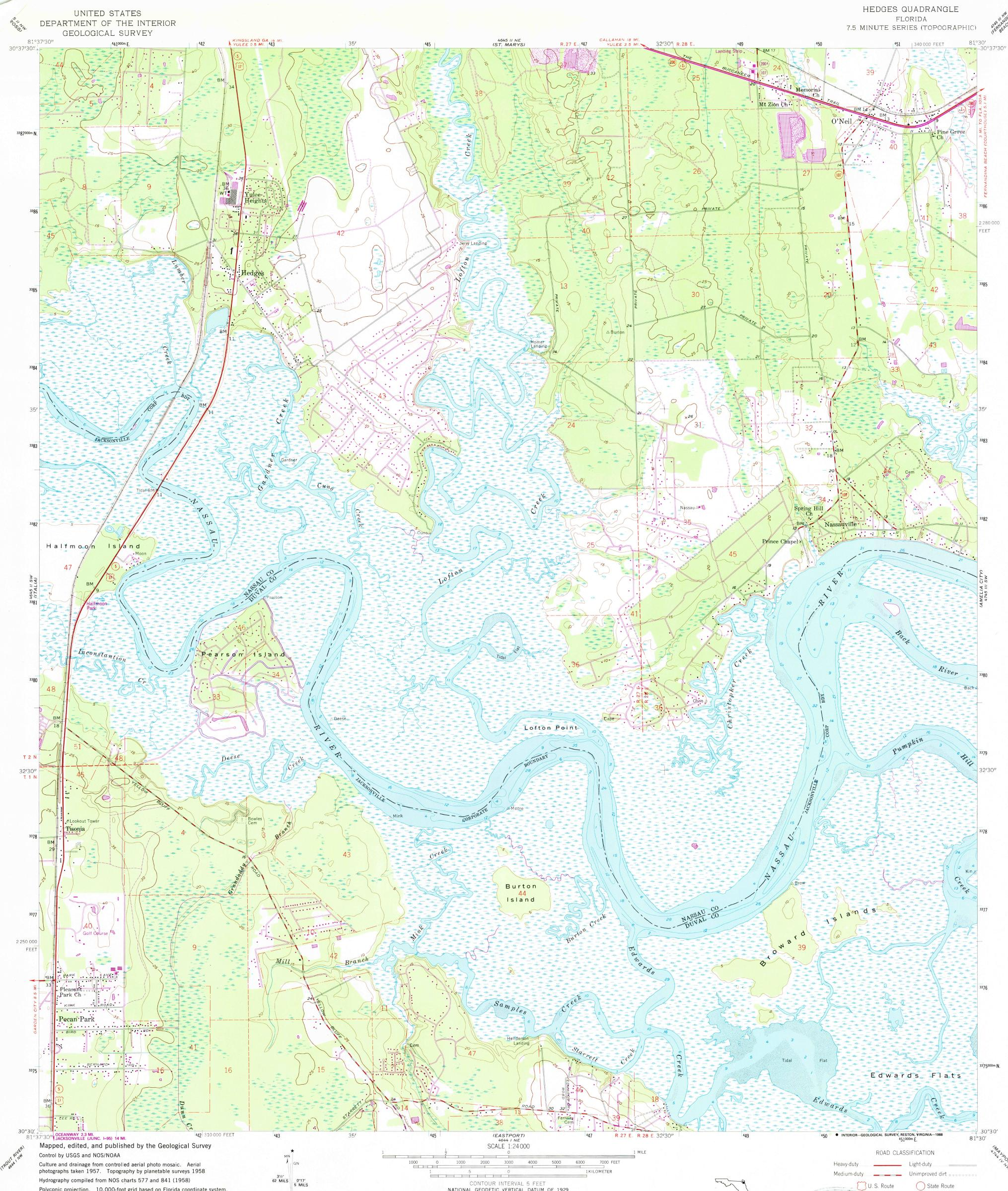
Polyconic projection. 10,000-foot grid based on Florida coordinate system, east zone. 1000-meter Universal Transverse Mercator grid ticks, zone 17, shown in blue. 1927 North American Datum. To place on the predicted North American Datum 1983 move the projection lines 21 meters south and 17 meters west as shown by dashed corner ticks
