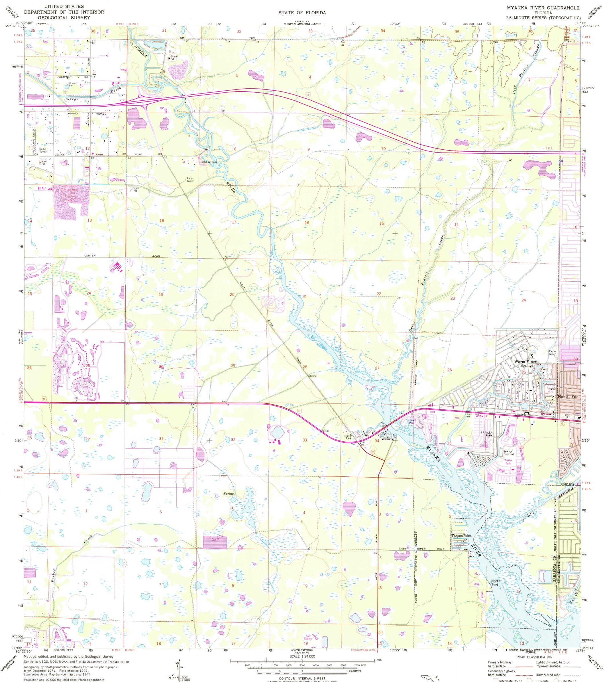
Projection and 10,000-foot grid ticks: Florida coordinate system, west zone (transverse Mercator) 1000-meter Universal Transverse Mercator grid ticks, zone 17, shown in blue 1927 North American datum To place on the predicted North American Datum 1983 move the projection lines 33 meters south and 16 meters west as shown by dashed corner ticks
