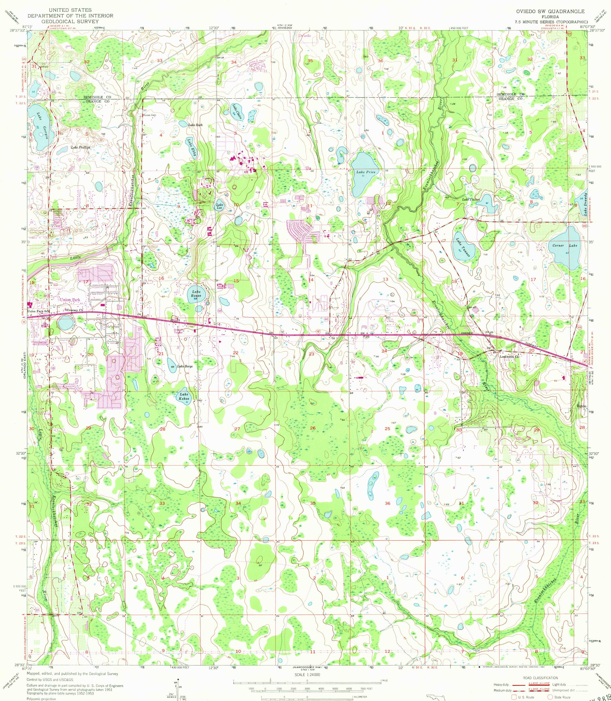
Polyconic projection 10,000-foot grid based on Florida coordinate system, east zone 1000-meter Universal Transverse Mercator grid ticks, zone 17, shown in blue. 1927 North American Datum To place on the predicted North American Datum 1983 move the projection lines 27 meters south and 19 meters west as shown by dashed corner ticks Revisions shown in purple compiled from aerial photographs taken 1977 and other source data. This information not field checked. Map edited 1980
