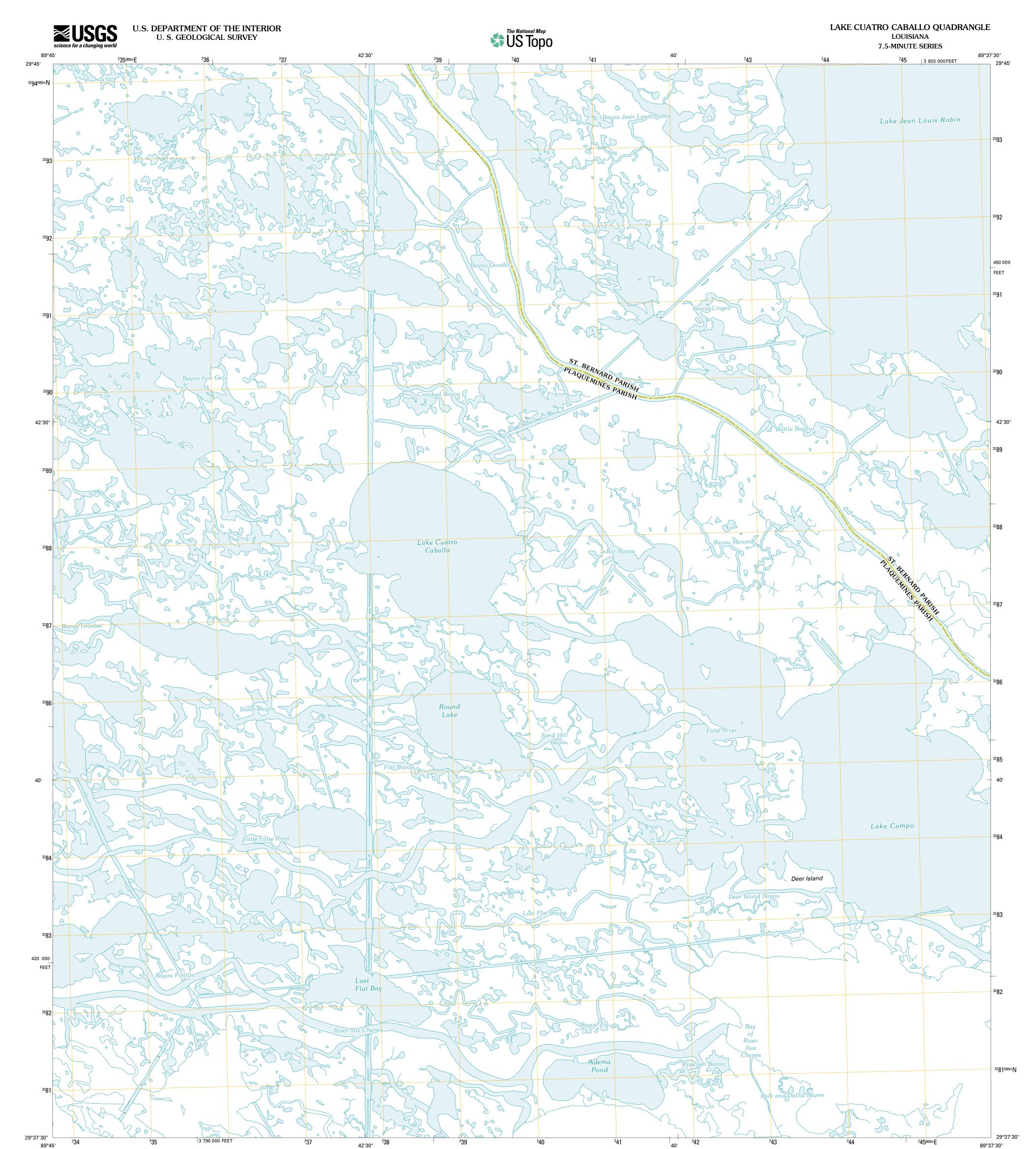
Produced by the United States Geological Survey North American Datum of 1983 (NAD83) World Geodetic System of 1984 (WGS84). Projection and 1 000-meter grid: Universal Transverse Mercator, Zone 16R 10 000-foot ticks: Louisiana Coordinate System of 1983 (couth 2002) (south zone)
