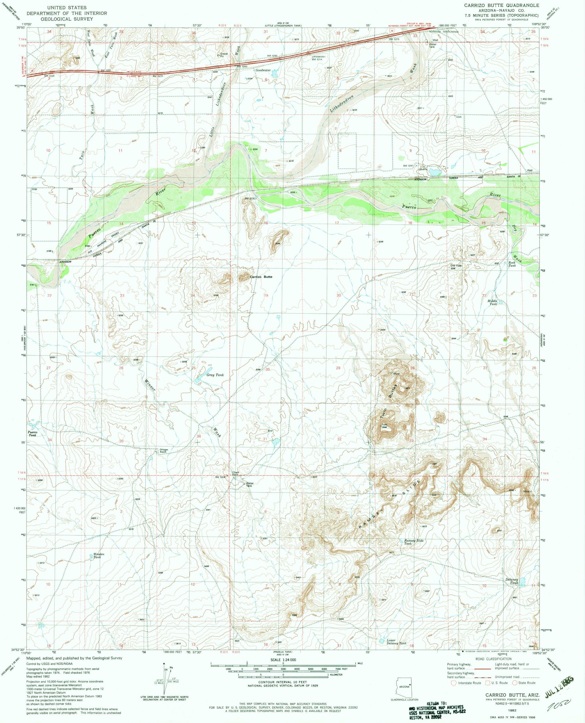
Projection and 10,000-foot grid ticks: Arizona coordinate system, east zone (transverse Mercator) 1000-meter Universal Transverse Mercator grid, zone 12 1927 North American Datum To place on the predicted North American Datum 1983 move the projection lines 60 meters east as shown by dashed corner ticks Fine red dashed lines indicate selected fence and field lines where
