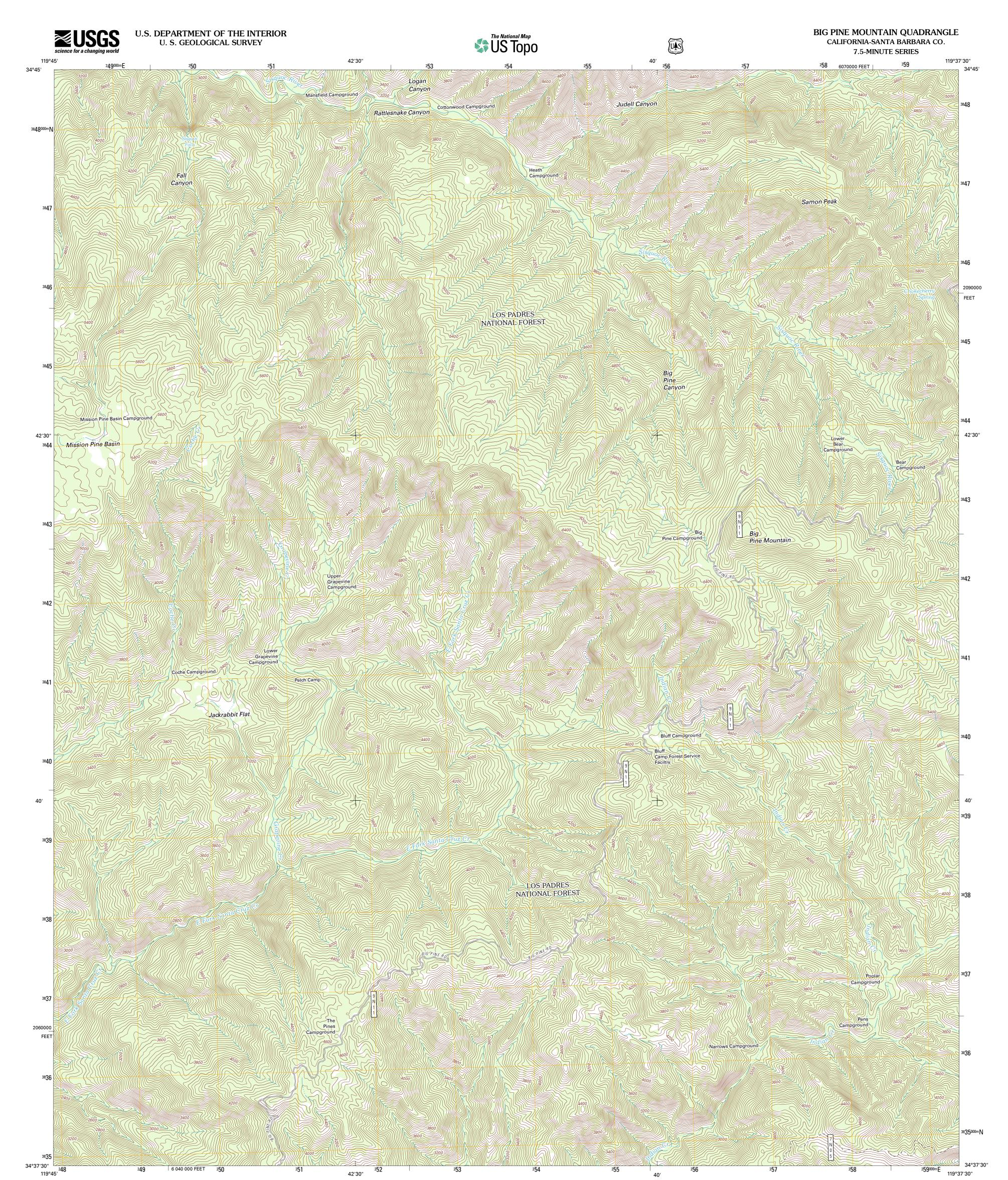
Produced by the United States Geological Survey North American Datum of 1983 (NAD83) World Geodetic System of 1984 (WGS84). Projection and 1 000-meter grid: Universal Transverse Mercator, Zone 11S 10 000-foot ticks: California Coordinate System of 1983 (zone 5) (zone 5)
