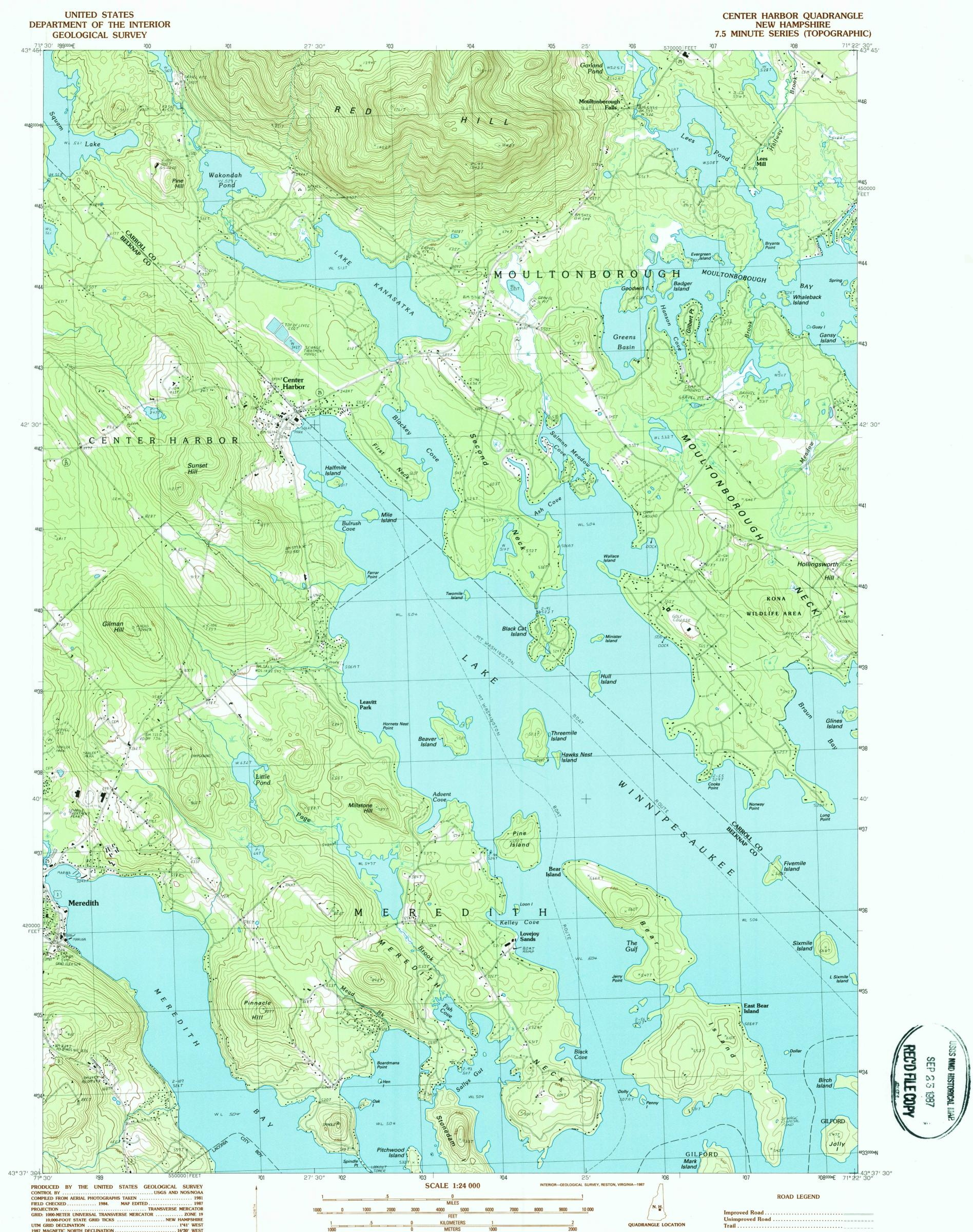
CONTROL ELEVATIONS SHOWN TO THE NEAREST 0.1 FOOT OTHER ELEVATIONS SHOWN TO THE NEAREST FOOT To convert feet to meters multiply by .3048 To convert meters to feet multiply by 3.2808 THIS MAP COMPLIES WITH NATIONAL MAP ACCURACY STANDARDS FOR SALE BY U. S. GEOLOGICAL SURVEY DENVER, COLORADO 80225, OR RESTON, VIRGINIA 22092
