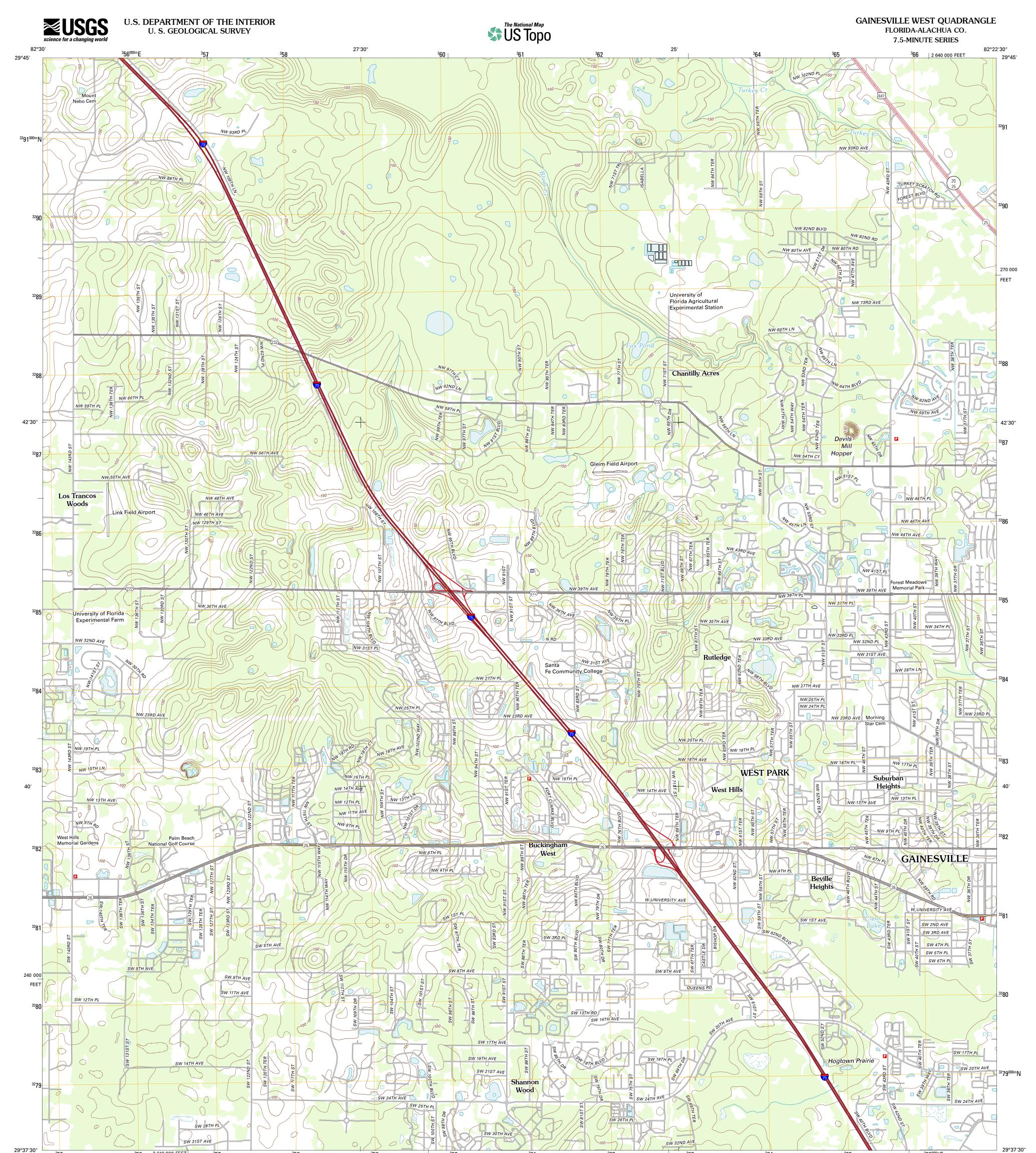
Produced by the United States Geological Survey North American Datum of 1983 (NAD83) World Geodetic System of 1984 (WGS84). Projection and 1 000-meter grid: Universal Transverse Mercator, Zone 17R 10 000-foot ticks: Florida Coordinate System of 1983 (north zone)
