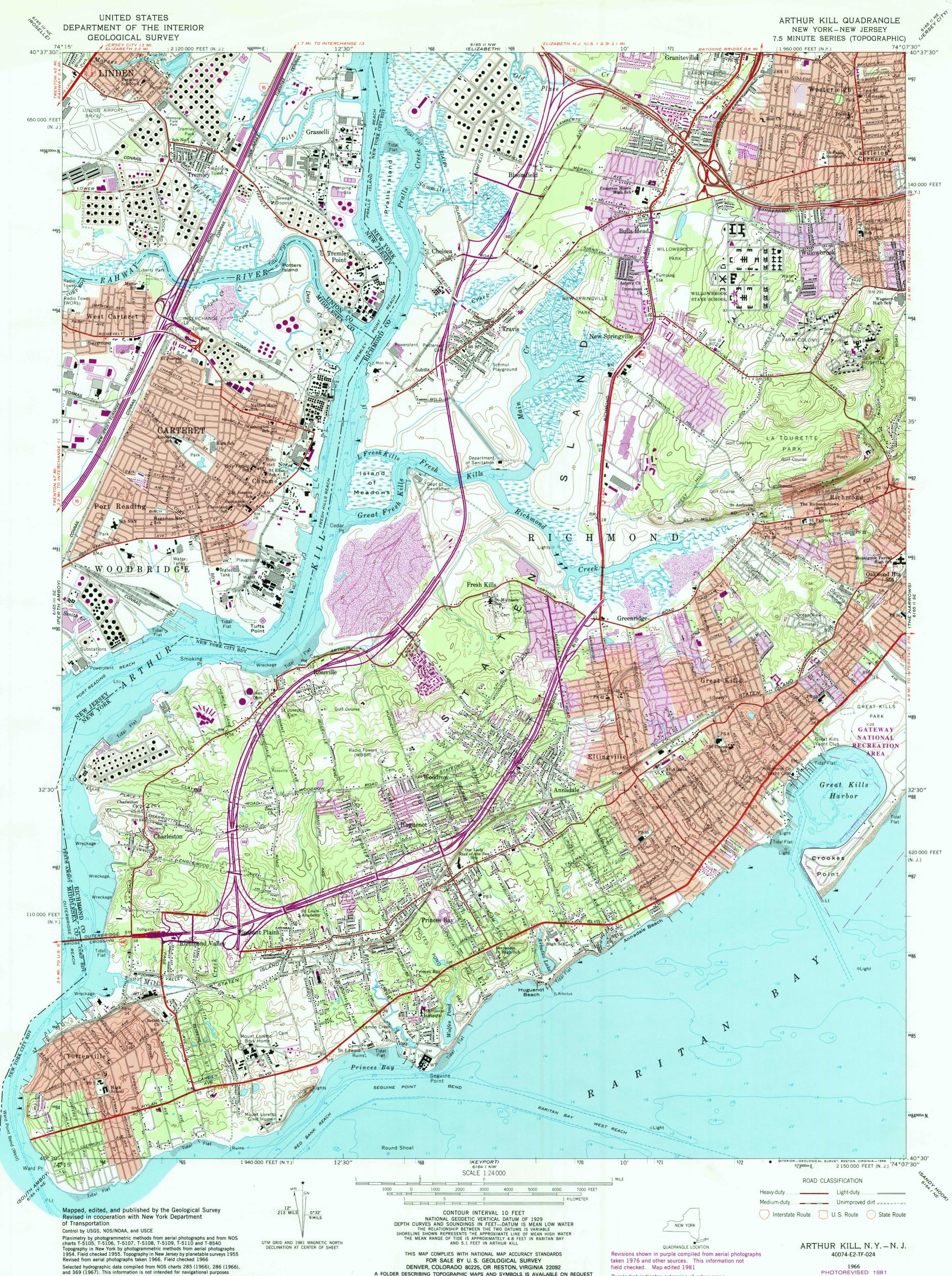
Polyconic projection. 10,000-foot grid ticks based on New York coordinate system, Long Island zone, and New Jersey coordinate system. 1000-meter Universal Transverse Mercator grid ticks, zone 18, shown in blue. 1927 North American Datum. To place on the predicted North American Datum 1983 move the projection lines 6 meters south and 34 meters west as shown by dashed corner ticks
