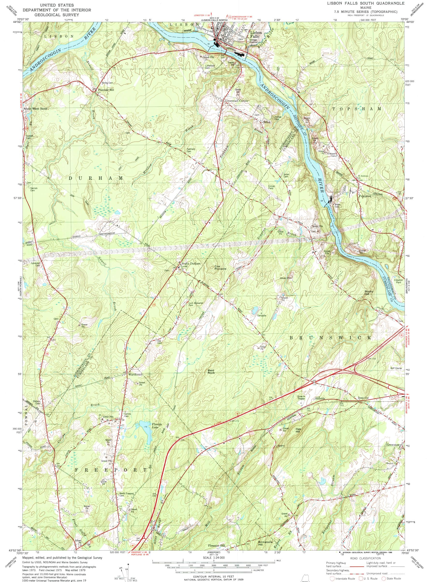
1000-meter Universal Transverse Mercator grid, zone 19 1927 North American datum To place on the predicted North American Datum 1983 move the projection lines 4 meters south and 42 meters west as shown by dashed corner ticks
