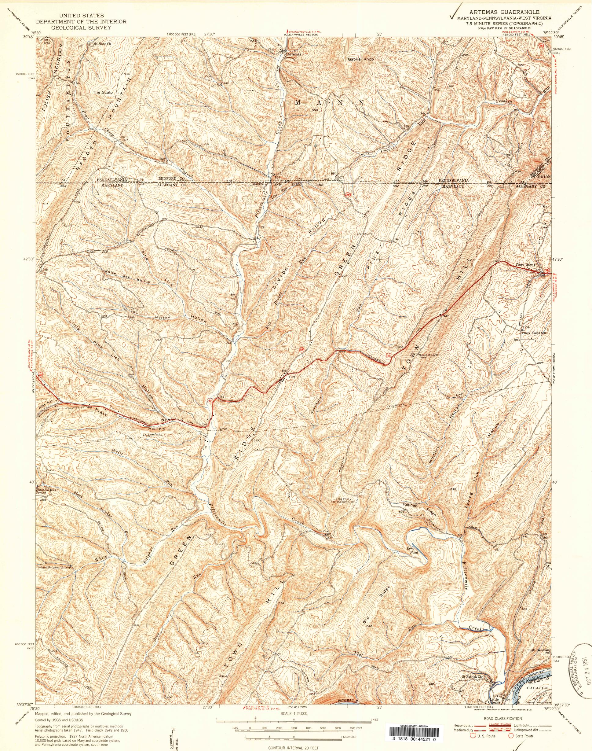
Polyconic projection. 1927 North American datum 10,000-foot grids based on Maryland coordinate system, and Pennsylvania coordinate system, south zone
