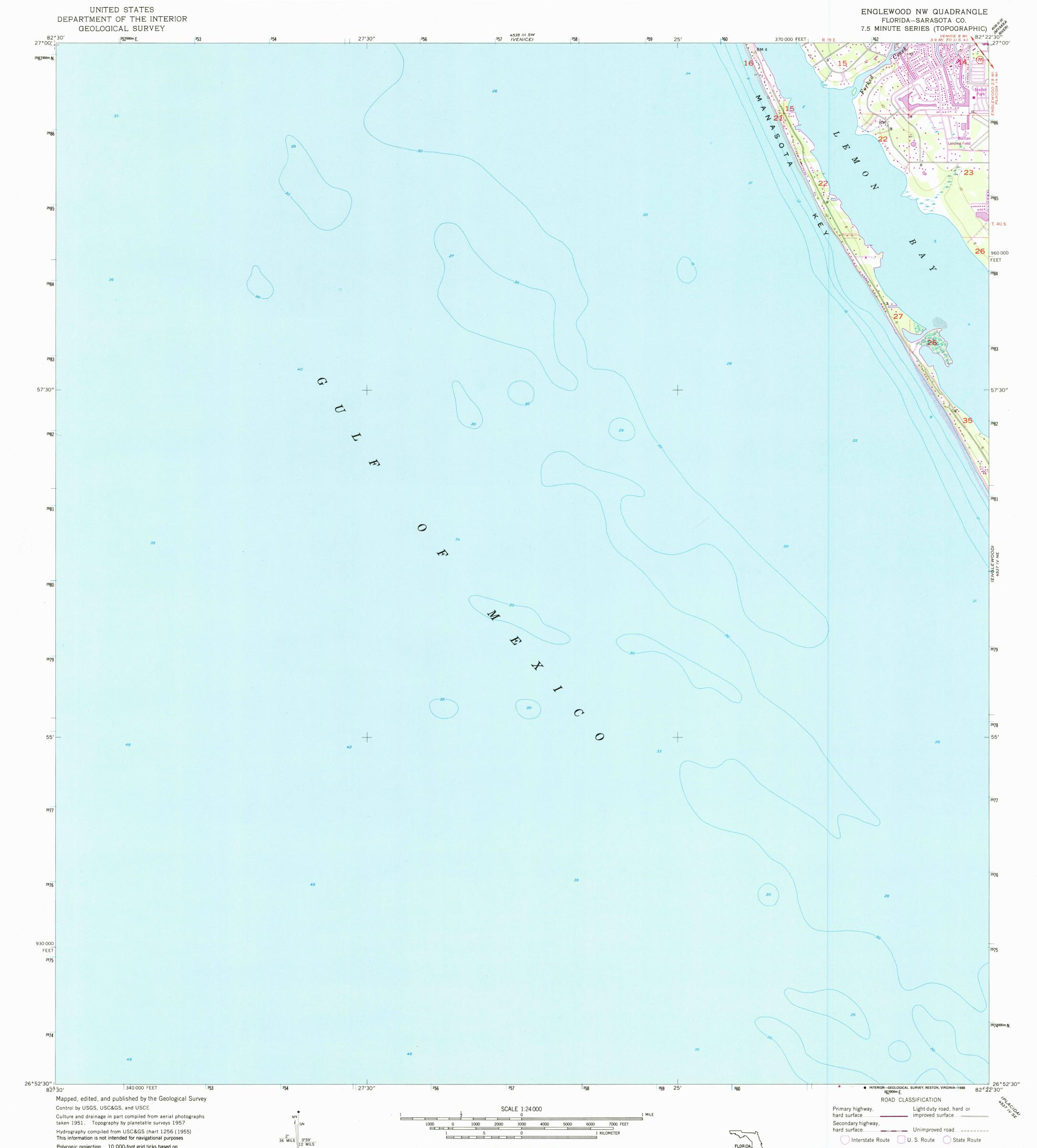
Polyconic projection. 10,000-foot grid ticks based on Florida coordinate system, west zone 1000-meter Universal Transverse Mercator grid ticks, zone 17, shown in blue 1927 North American Datum To place on the predicted North American Datum 1983 move the projection lines 33 meters south and 16 meters west as shown by dashed corner ticks Dashed land lines indicate approximate locations
