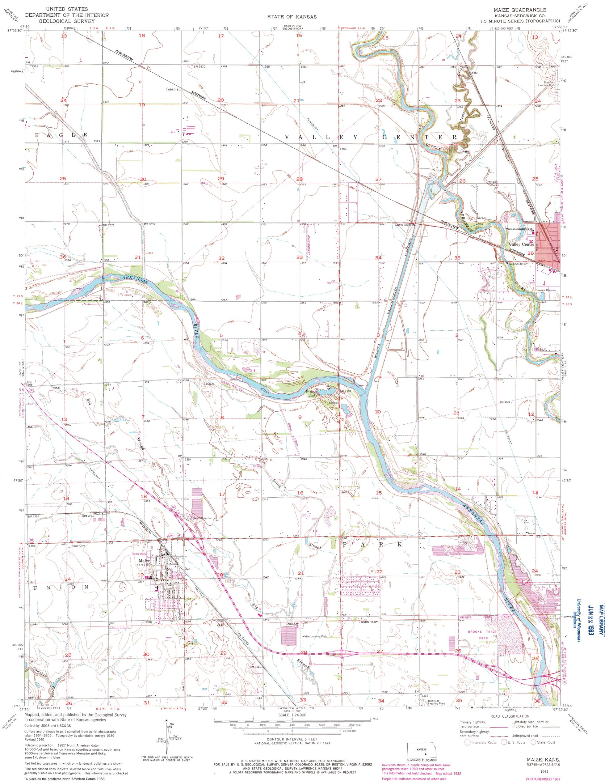
To place on the predicted North American Datum 1983 move the projection lines 28 meters east as shown by dashed corner ticks
