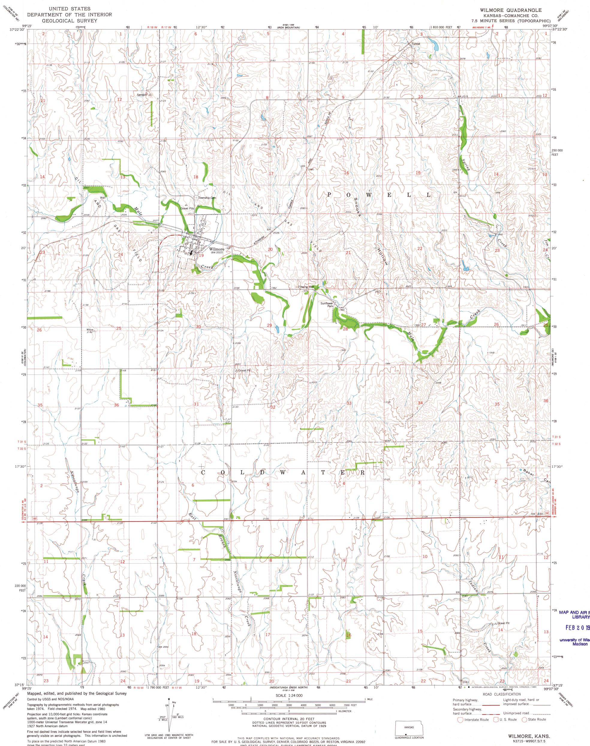
move the projection lines 33 meters east as shown by dashed corner ticks
