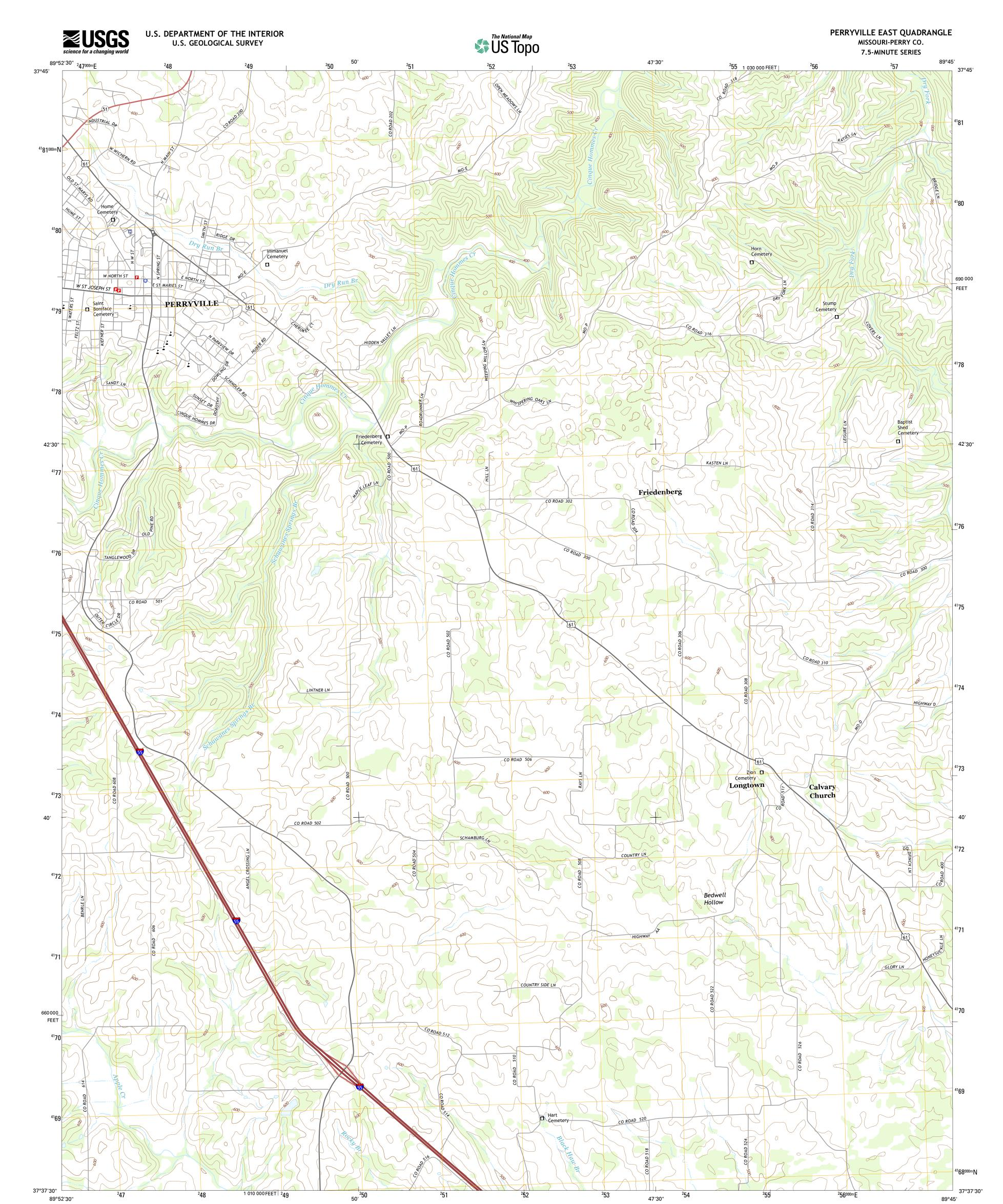
Produced by the United States Geological Survey North American Datum of 1983 (NAD83) World Geodetic System of 1984 (WGS84). Projection and 1 000-meter grid: Universal Transverse Mercator, Zone 165 10 000-foot ticks: Missouri Coordinate System of 1983 (east zone)
