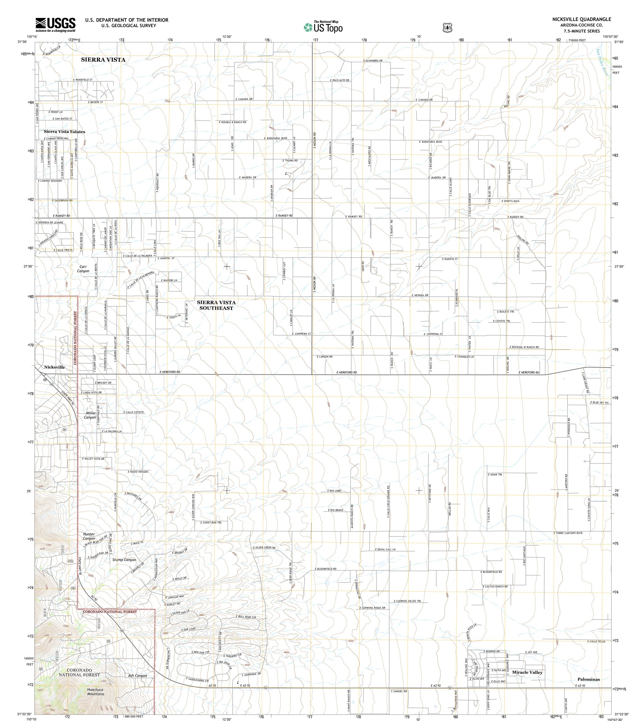
Produced by the United States Geological Survey North American Datum of 1983 (NAD83) World Geodetic System of 1984 (WGS84). Projection and 1 000-meter grid: Universal Transverse Mercator, Zone 12R 10 000-foot ticks: Arizona Coordinate System of 1983 (east zone)
