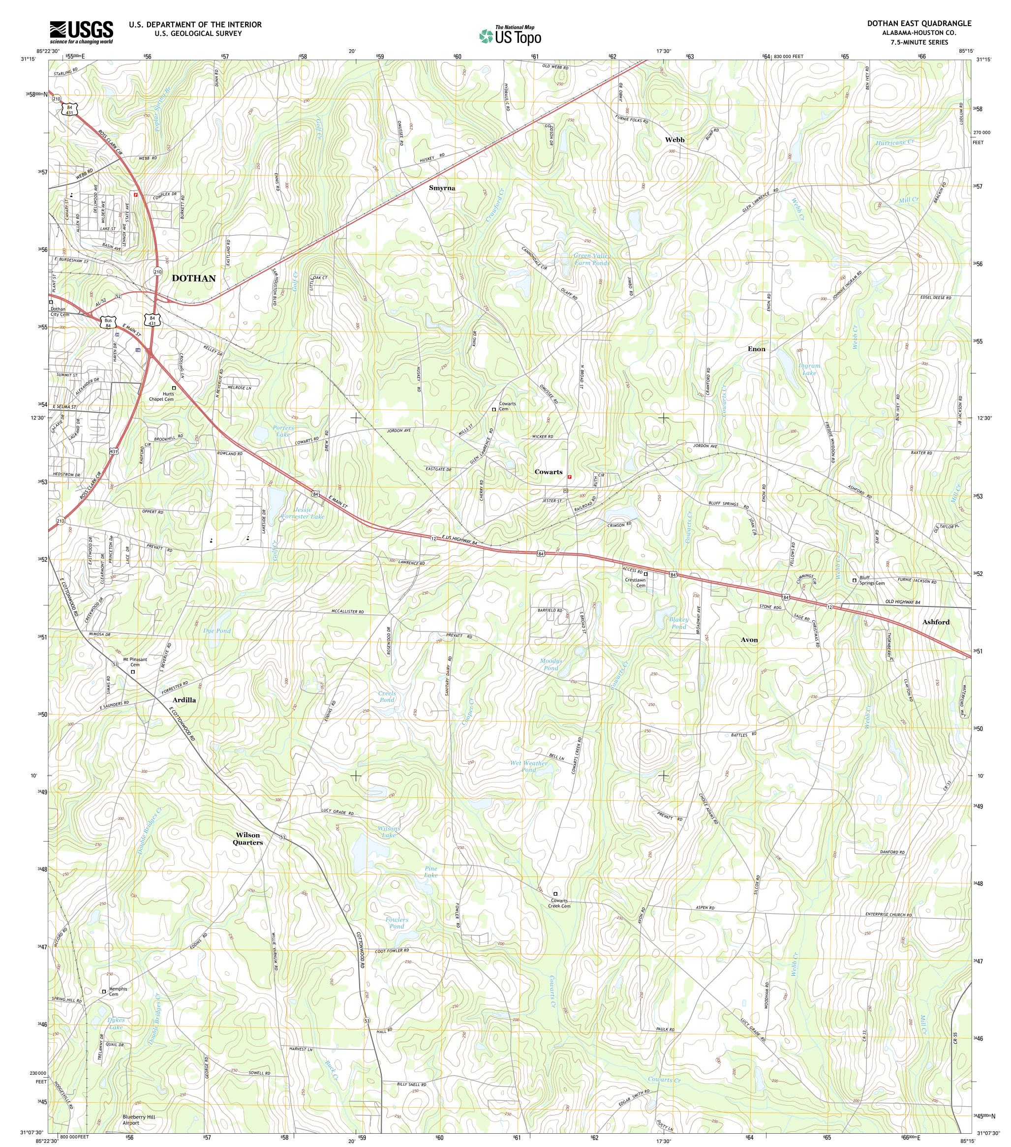
Produced by the United States Geological Survey North American Datum of 1983 (NAD83) World Geodetic System of 1984 (WGS84). Projection and 1 000-meter grid: Universal Transverse Mercator, Zone 16R 10 000-foot ticks: Alabama Coordinate System of 1983 (east zone)
