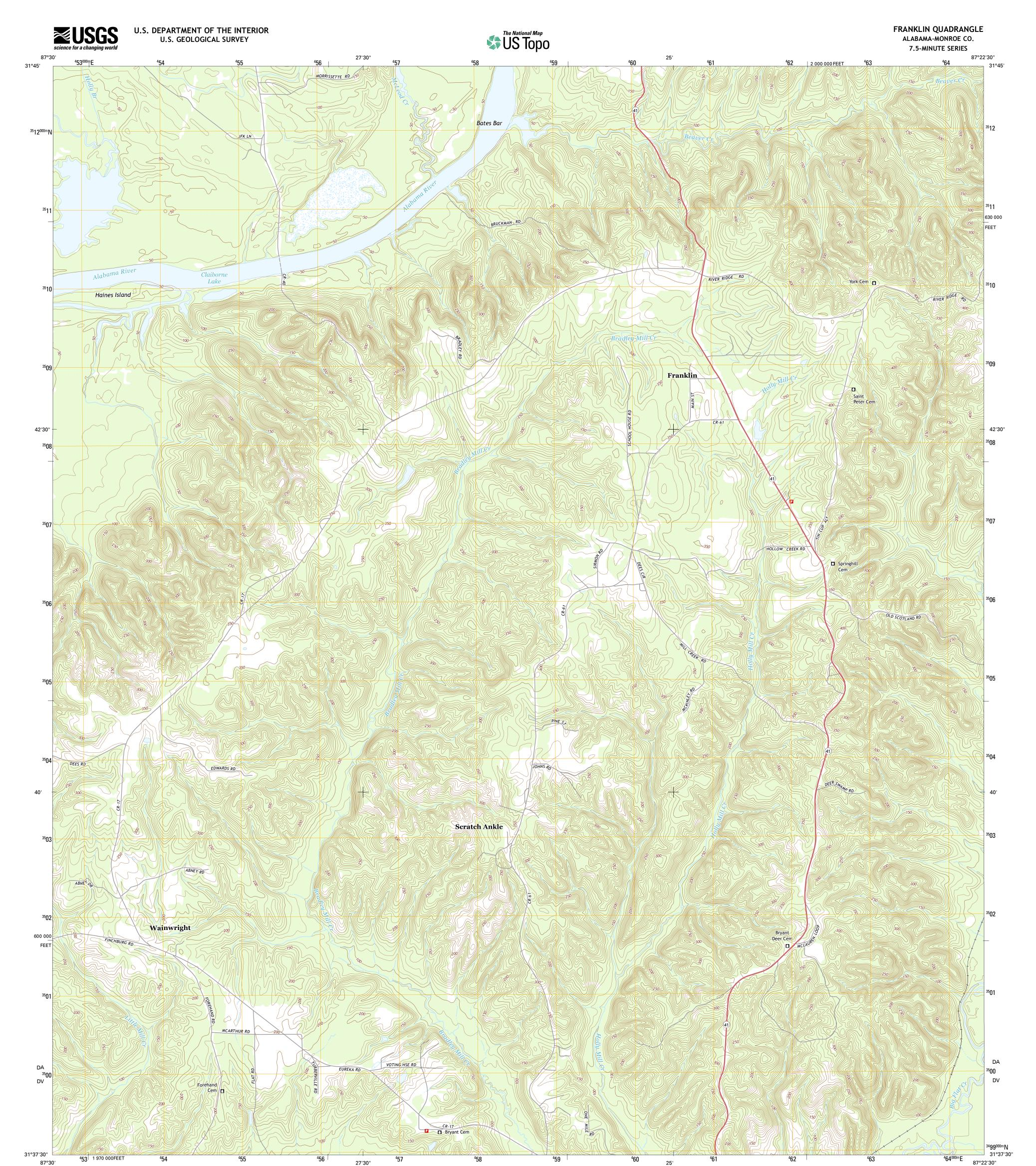
Produced by the United States Geological Survey North American Datum of 1983 (NAD83) World Geodetic System of 1984 (WGS84). Projection and 1 000-meter grid: Universal Transverse Mercator, Zone 16R 10 000-foot ticks: Alabama Coordinate System of 1983 (west zone)
