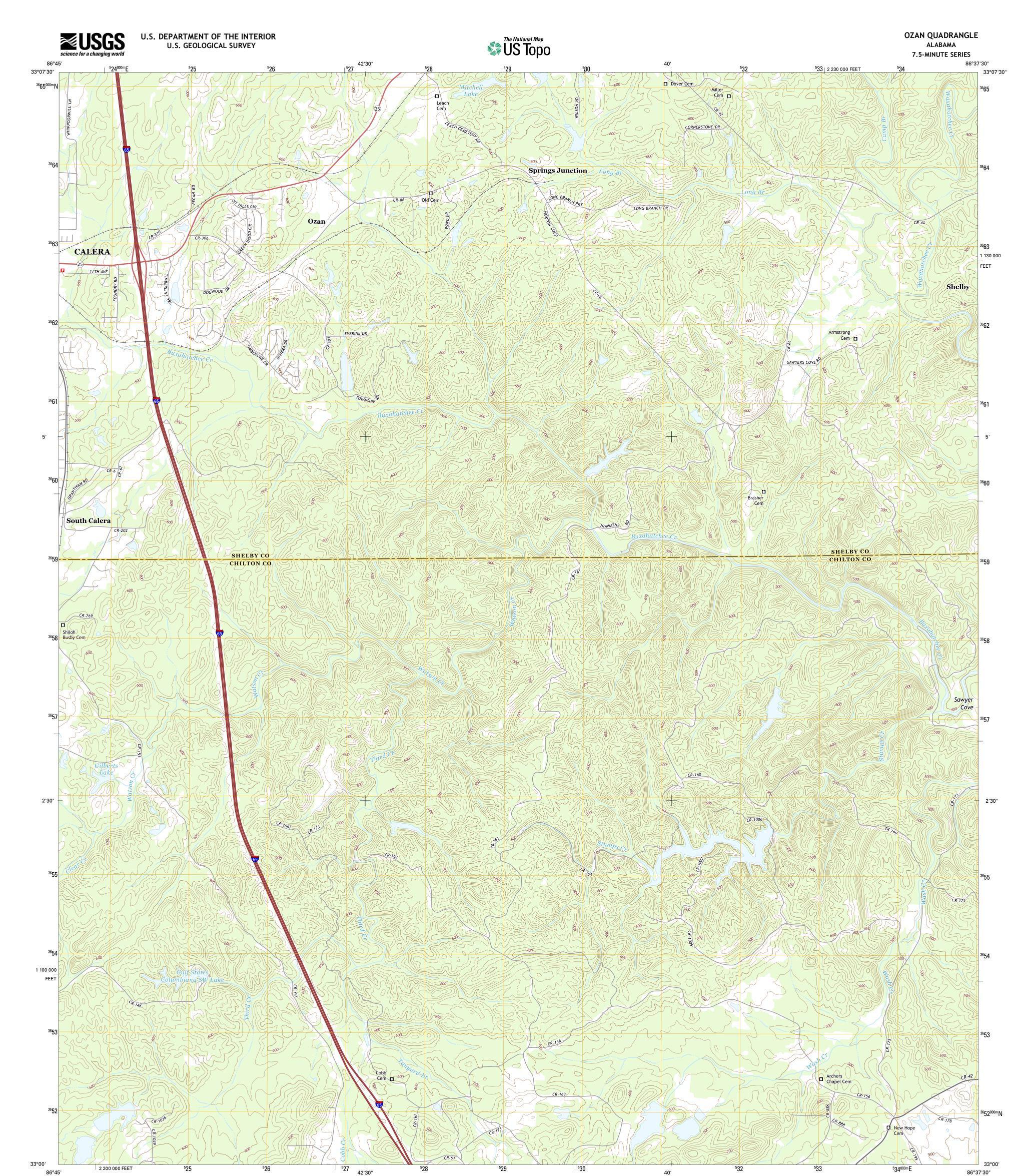
Produced by the United States Geological Survey North American Datum of 1983 (NAD83) World Geodetic System of 1984 (WGS84). Projection and 1 000-meter grid: Universal Transverse Mercator, Zone 16S 10 000-foot ticks: Alabama Coordinate System of 1983 (west Zone) zone)
