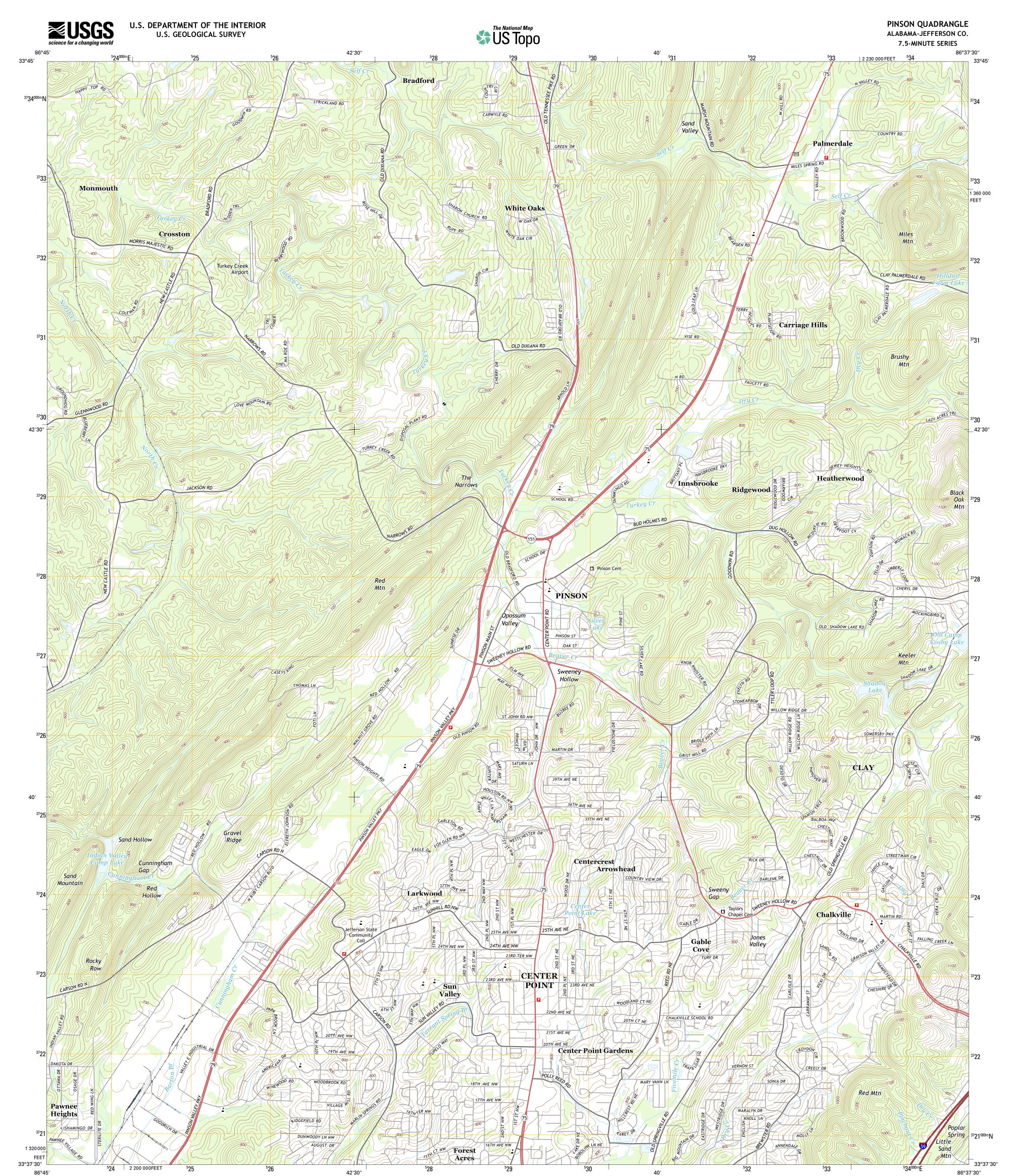
Produced by the United States Geological Survey North American Datum of 1983 (NAD83) World Geodetic System of 1984 (WGS84). Projection and 1 000-meter grid: Universal Transverse Mercator, Zone 165 10 000-foot ticks: Alabama Coordinate System of 1983 (west zone)
