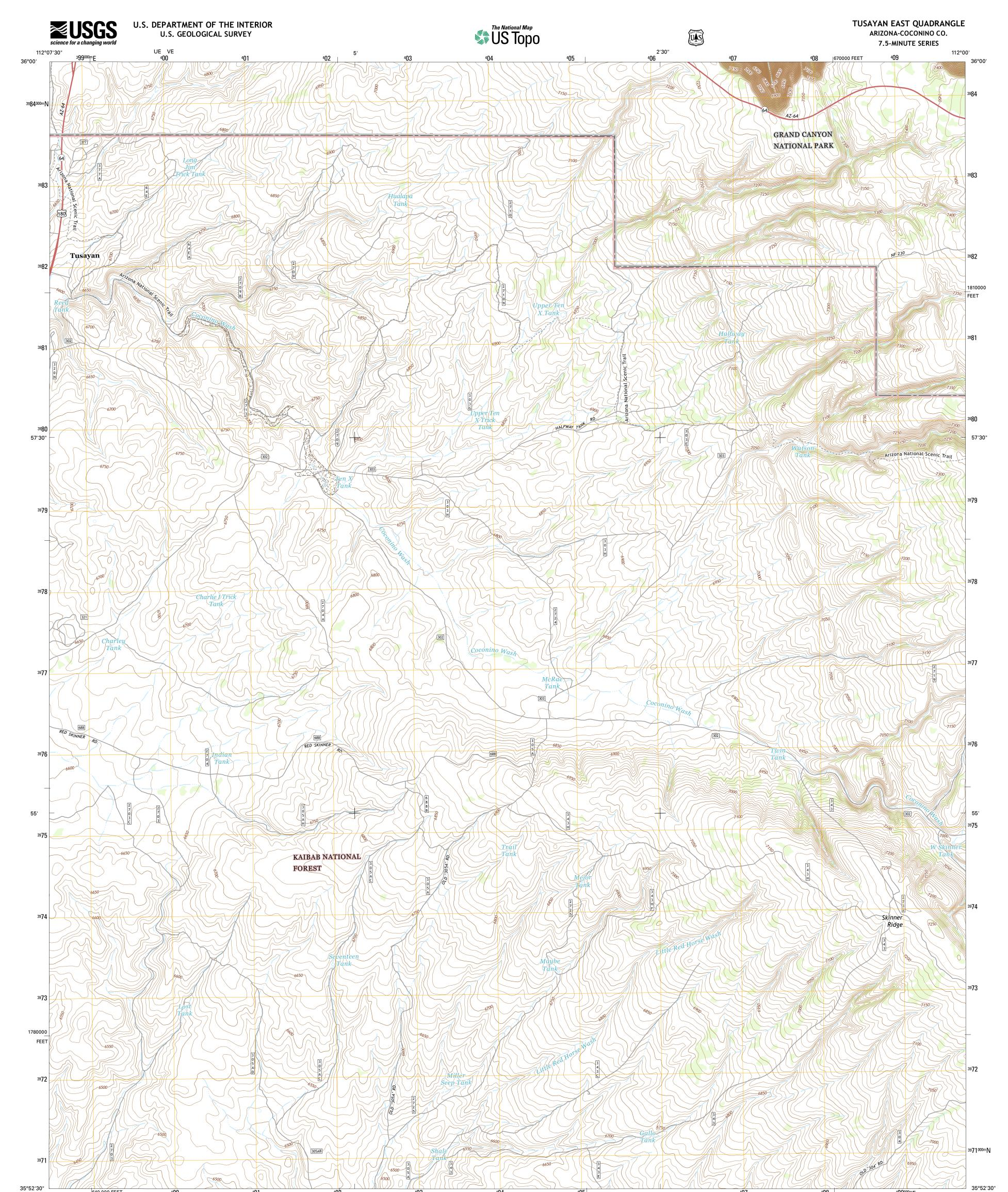
Produced by the United States Geological Survey North American Datum of 1983 (NAD83) World Geodetic System of 1989 (WGS84). Projection and 1 000-meter grid: Universal Transverse Mercator, Zone 12S 10 000-foot ticks: Arizona Coordinate System of 1983 (central zone)
