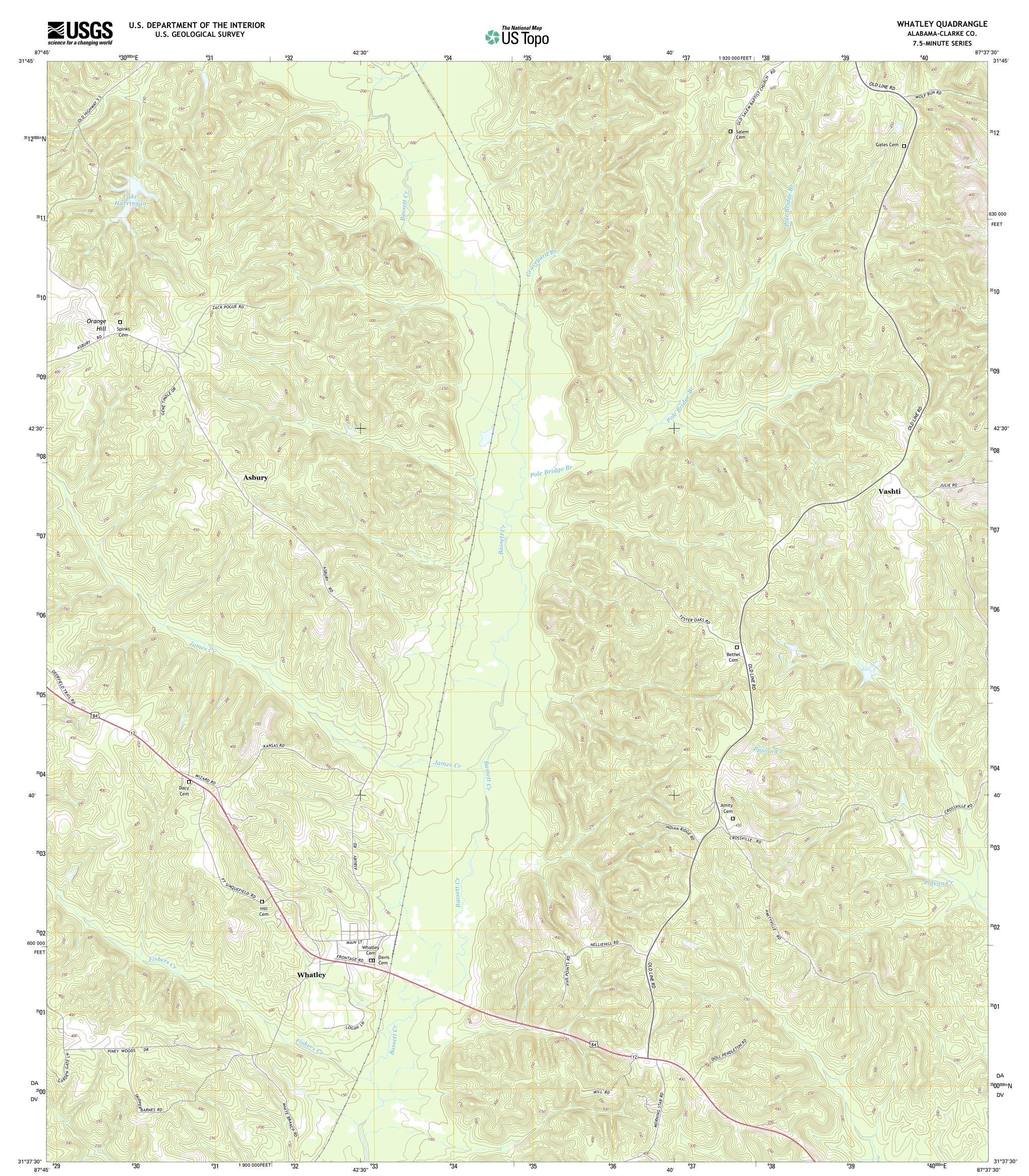
Produced by the United States Geological Survey North American Datum of 1983 (NAD83) World Geodetic System of 1984 (WGS84). Projection and 1 000-meter grid: Universal Transverse Mercator, Zone 16R 10 000-foot ticks: Alabama Coordinate System of 1983 (west Zone) zone)
