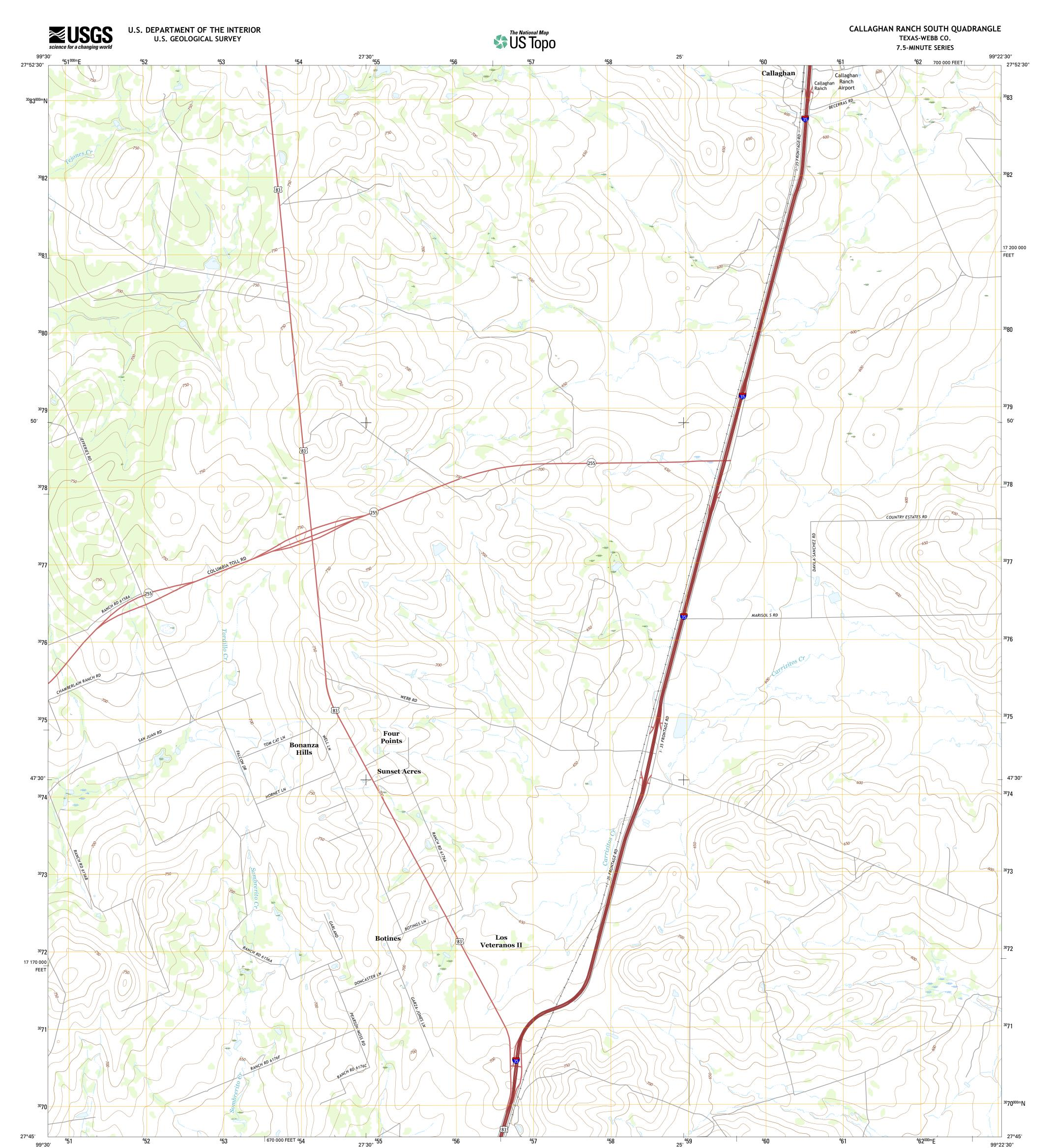
Produced by the United States Geological Survey North American Datum of 1983 (NAD83) World Geodetic System of 1984 (WGS84). Projection and 1 000-meter grid: Universal Transverse Mercator, Zone 14R 10 000-foot ticks: Texas Coordinate System of 1983 (south zone)
