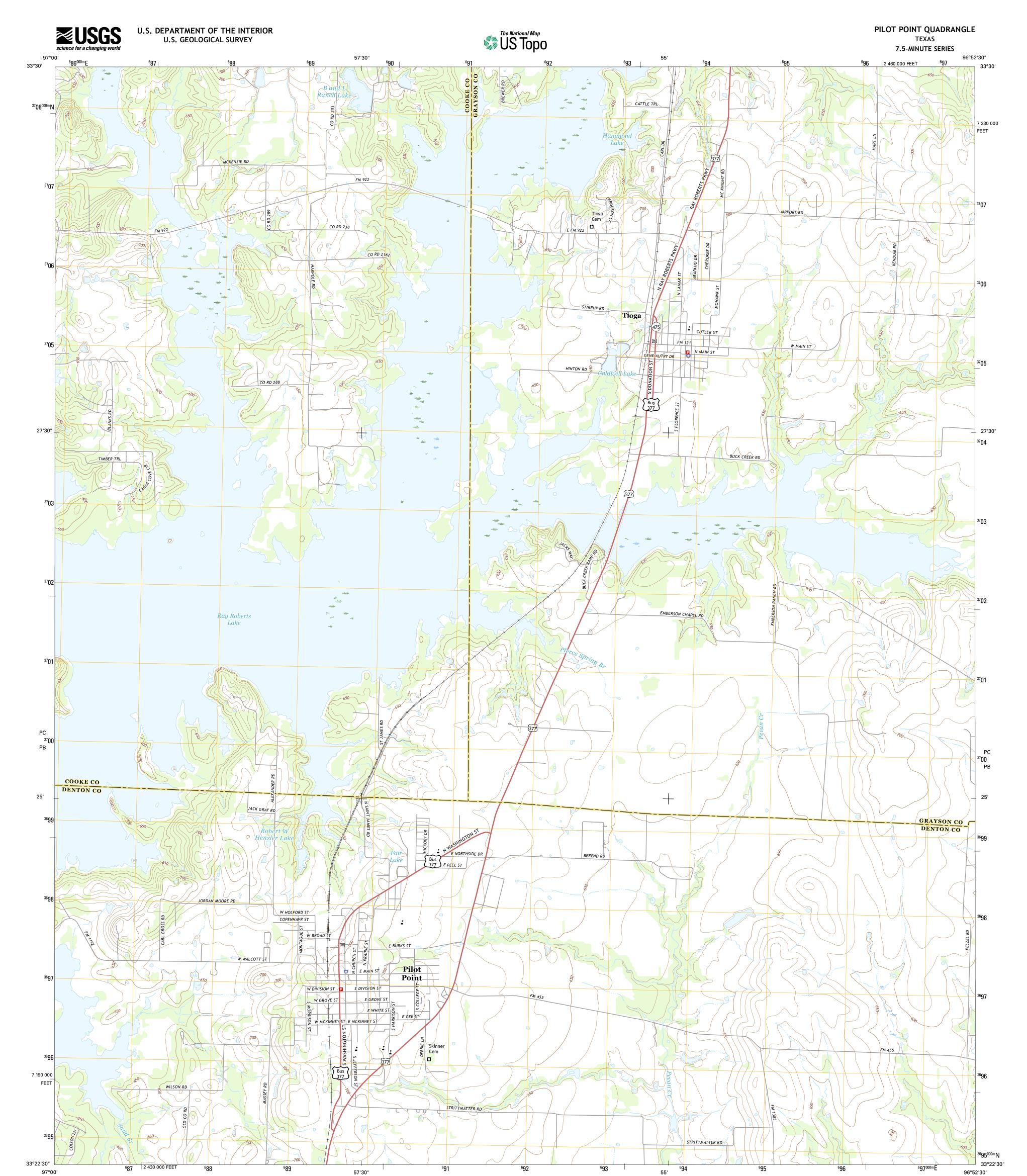
**Produced by the United States Geological Survey** North American Datum of 1983 (NAD83) World Geodetic System of 1984 (WGS84). Projection and 1 000-meter grid: Universal Transverse Mercator, Zone 14S 10 000-foot ticks: Texas Coordinate System of 1983 (north central zone) central zone)
