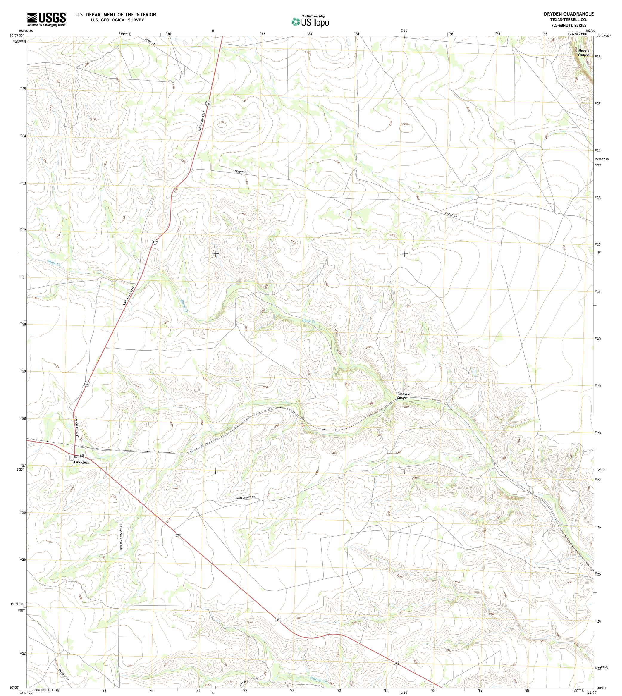
Produced by the United States Geological Survey North American Datum of 1983 (NAD83) World Geodetic System of 1984 (WGS84). Projection and 1 000-meter grid: Universal Transverse Mercator, Zone 13R 10 000-foot ticks: Texas Coordinate System of 1983 (south central zone)
