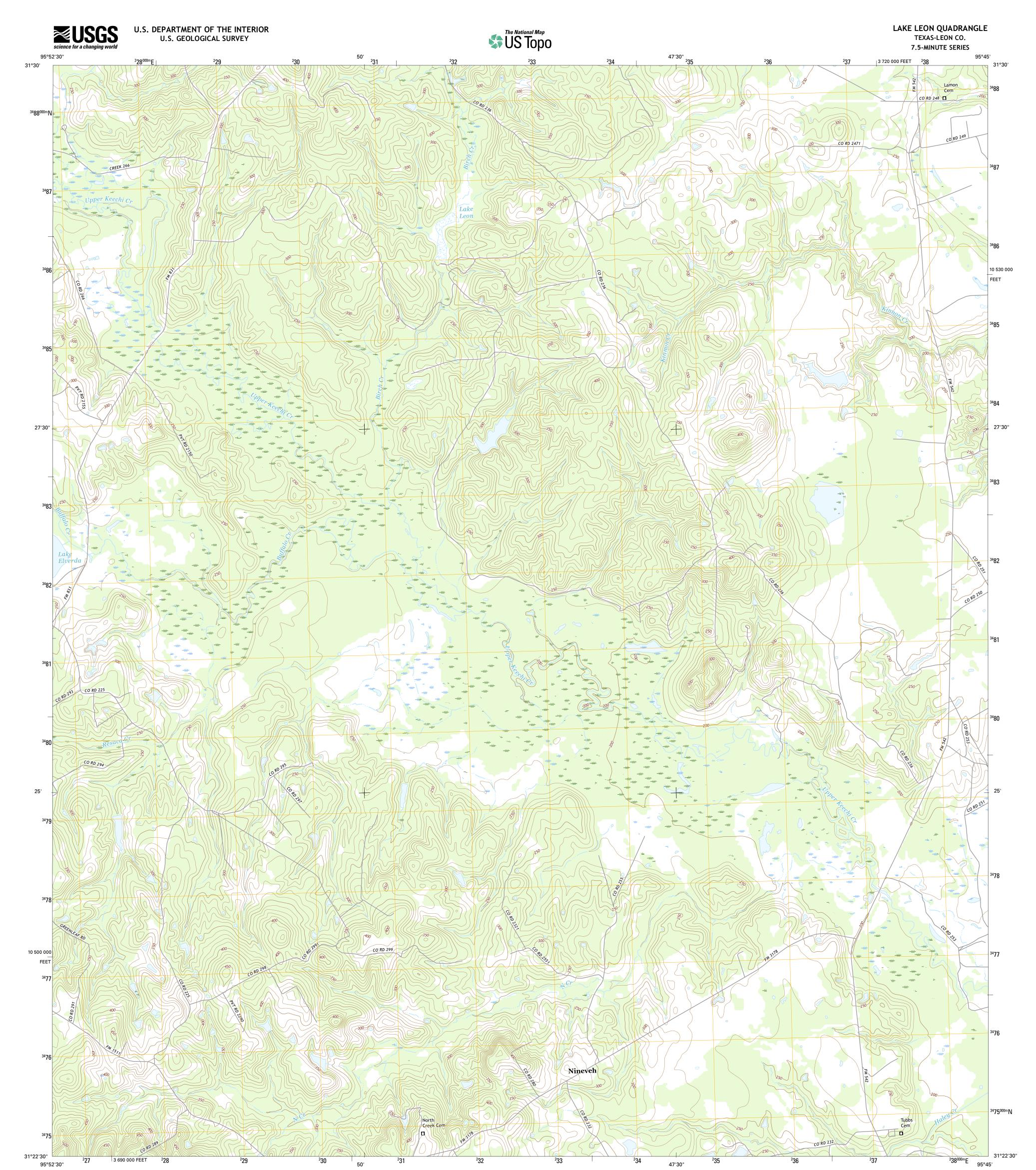
**Produced by the United States Geological Survey** North American Datum of 1983 (NAD83) World Geodetic System of 1984 (WGS84). Projection and 1 000-meter grid: Universal Transverse Mercator, Zone 15R 10 000-foot ticks: Texas Coordinate System of 1983 (central zone)
