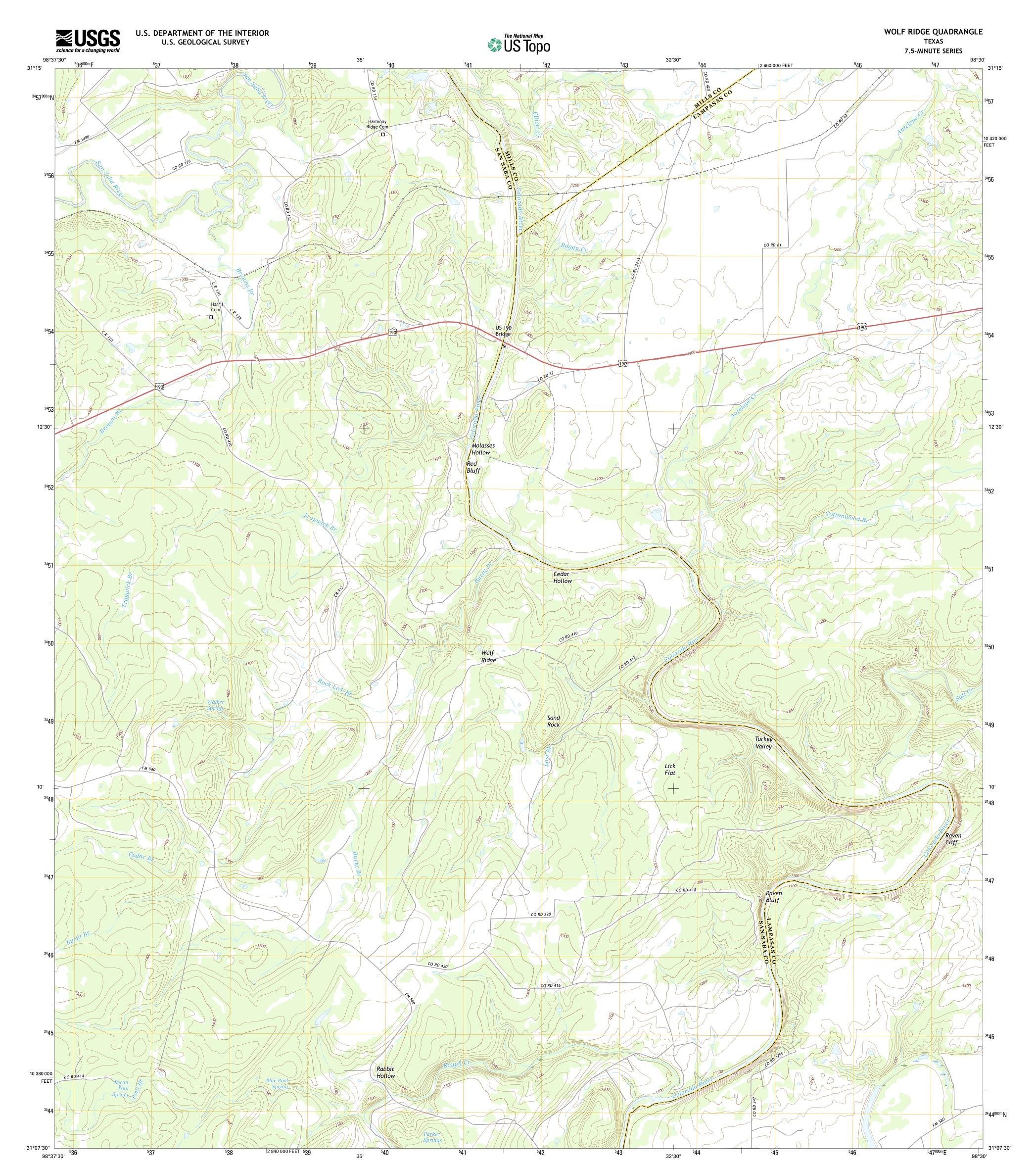
Produced by the United States Geological Survey North American Datum of 1983 (NAD83) World Geodetic System of 1984 (WGS84). Projection and 1 000-meter grid: Universal Transverse Mercator, Zone 14R 10 000-foot ticks: Texas Coordinate System of 1983 (central zone)
