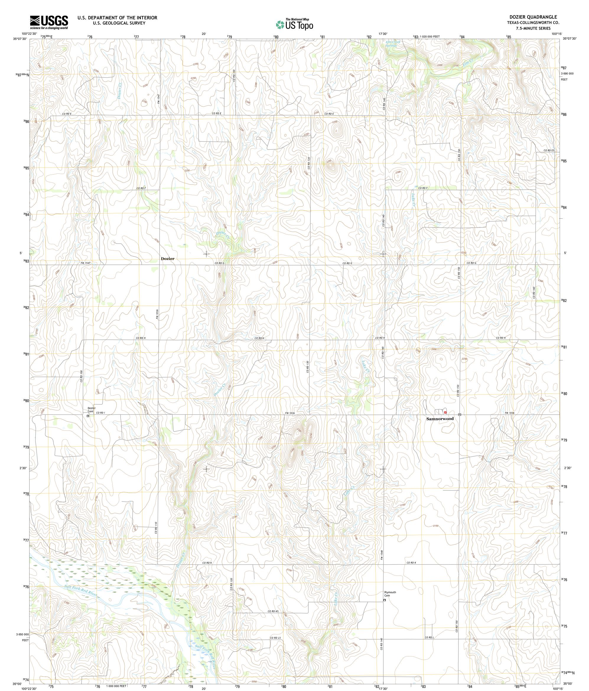
100°22'30" Produced by the United States Geological Survey North American Datum of 1983 (NAD83) World Geodetic System of 1984 (WGS84). Projection and 1 000-meter grid: Universal Transverse Mercator, Zone 14S 10 000-foot ticks: Texas Coordinate System of 1983 (north zone)
