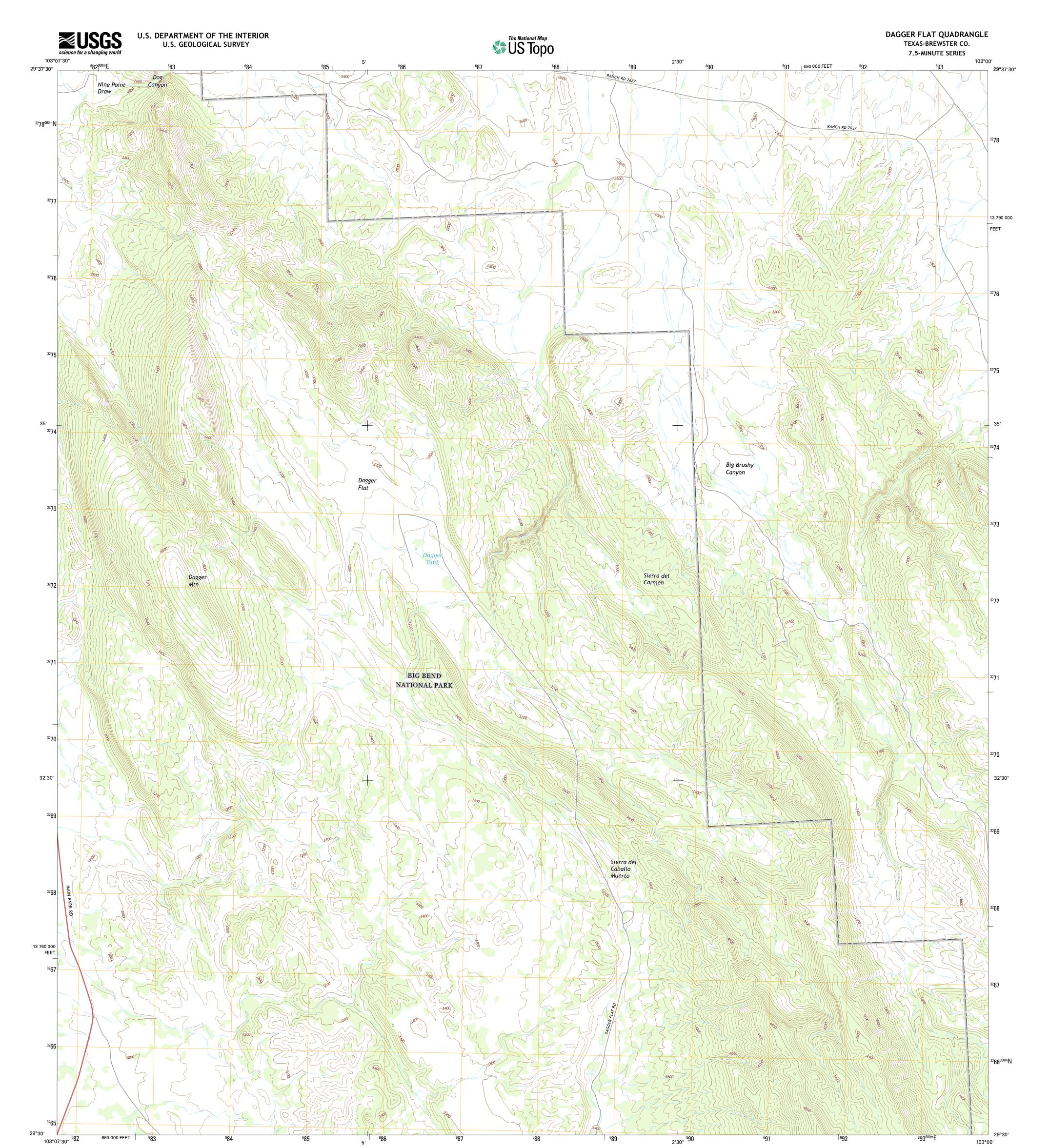
Produced by the United States Geological Survey North American Datum of 1983 (NAD83) World Geodetic System of 1984 (WGS84). Projection and 1 000-meter grid: Universal Transverse Mercator, Zone 13R 10 000-foot ticks: Texas Coordinate System of 1983 (south central zone) central zone)
