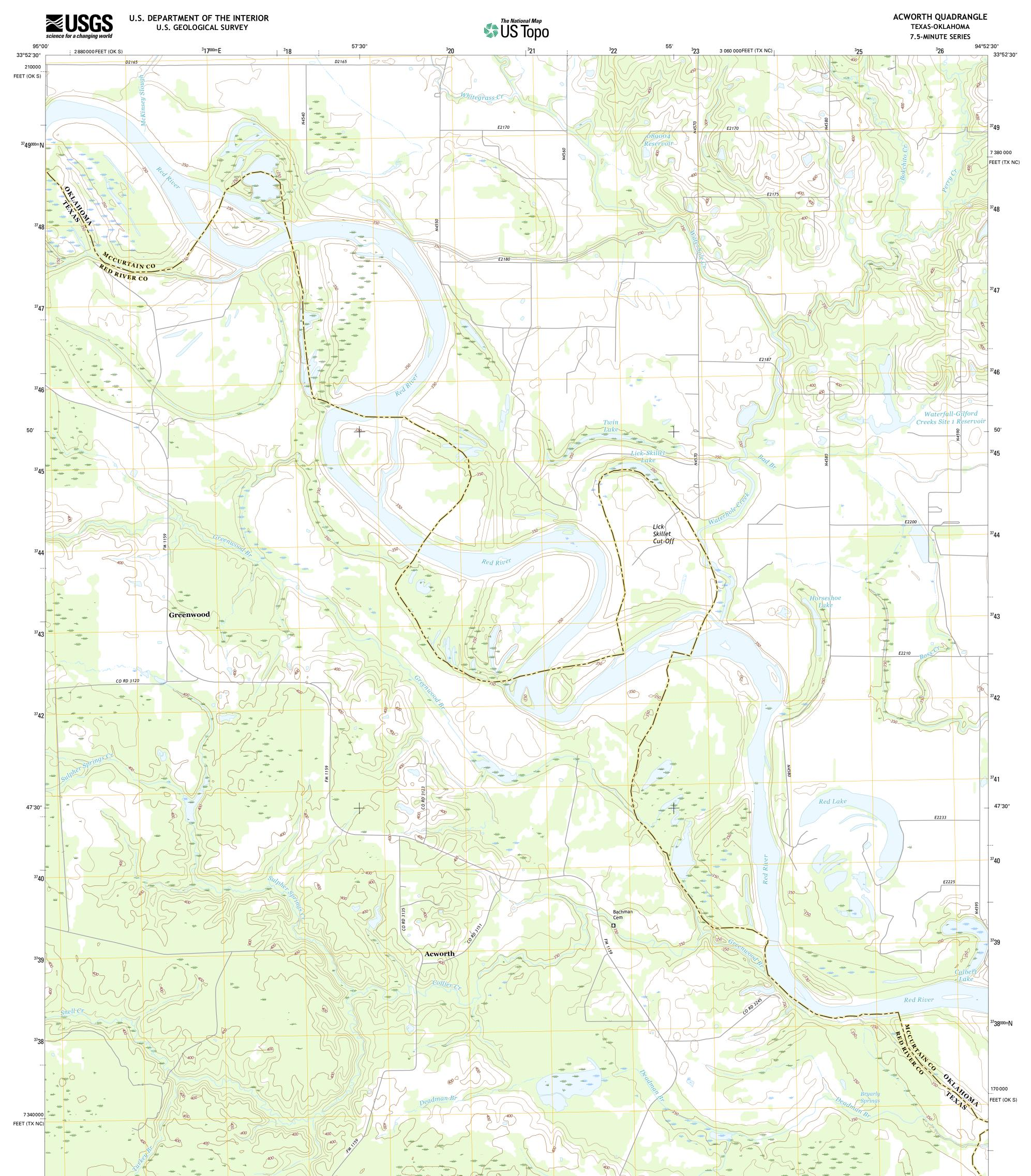
Produced by the United States Geological Survey North American Datum of 1983 (NAD83) World Geodetic System of 1984 (WGS84). Projection and 1 000-meter grid: Universal Transverse Mercator, Zone 15S 10 000-foot ticks: Texas Coordinate System of 1983 (north central zone), Oklahoma Coordinate System of 1983 (south Zone) zone)
