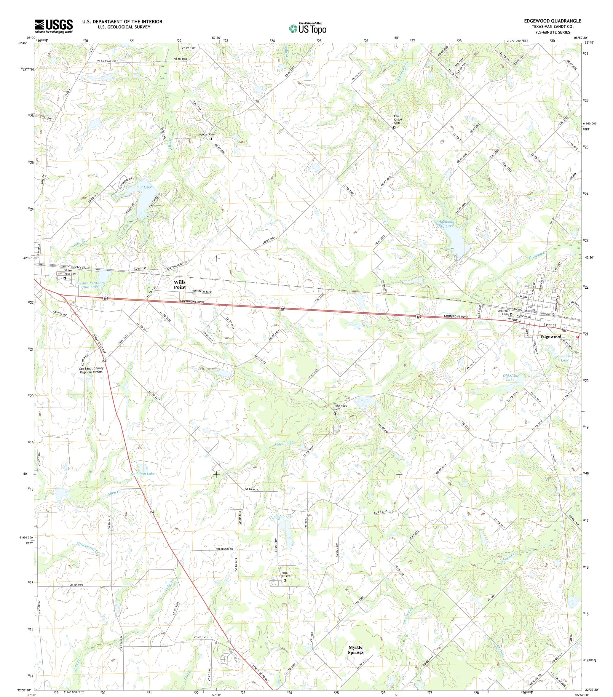
**Produced by the United States Geological Survey** North American Datum of 1983 (NAD83) World Geodetic System of 1984 (WGS84). Projection and 1 000-meter grid: Universal Transverse Mercator, Zone 15S 10 000-foot ticks: Texas Coordinate System of 1983 (north central zone) central zone)
