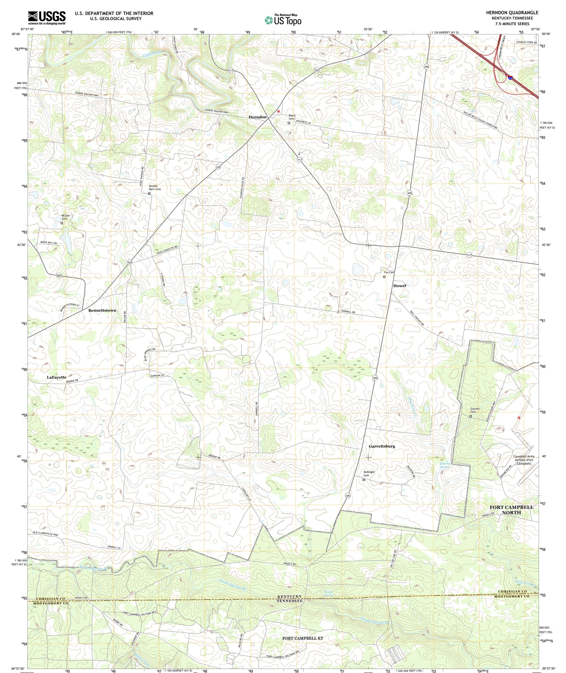
Produced by the United States Geological Survey North American Datum of 1983 (NAD83) World Geodetic System of 1984 (WGS84). Projection and 1 000-meter grid: Universal Transverse Mercator, Zone 16S 10 000-foot ticks: Kentucky Coordinate System of 1983 (south zone), Tennessee Coordinate System of 1983
