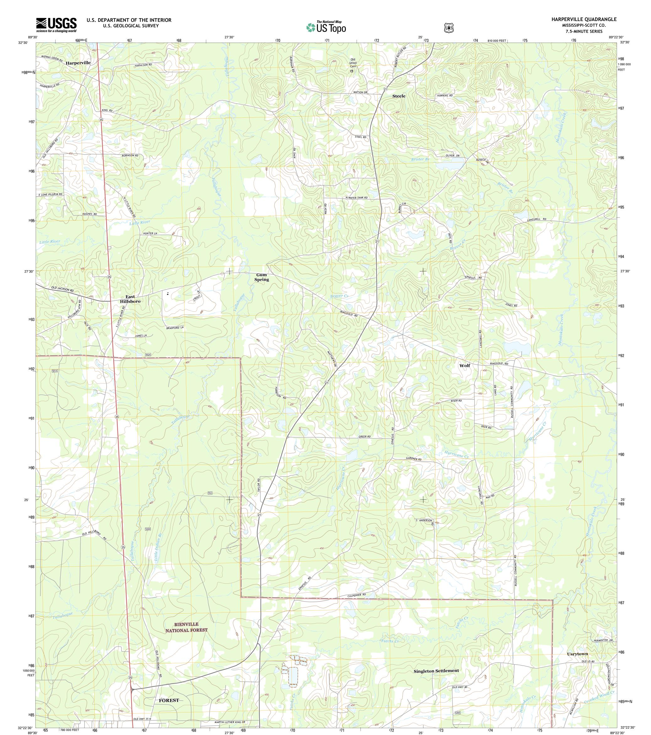
Produced by the United States Geological Survey North American Datum of 1983 (NAD83) World Geodetic System of 1984 (WGS84). Projection and 1 000-meter grid: Universal Transverse Mercator, Zone 16S 10 000-foot ticks: Mississippi Coordinate System of 1983 (east zone)
