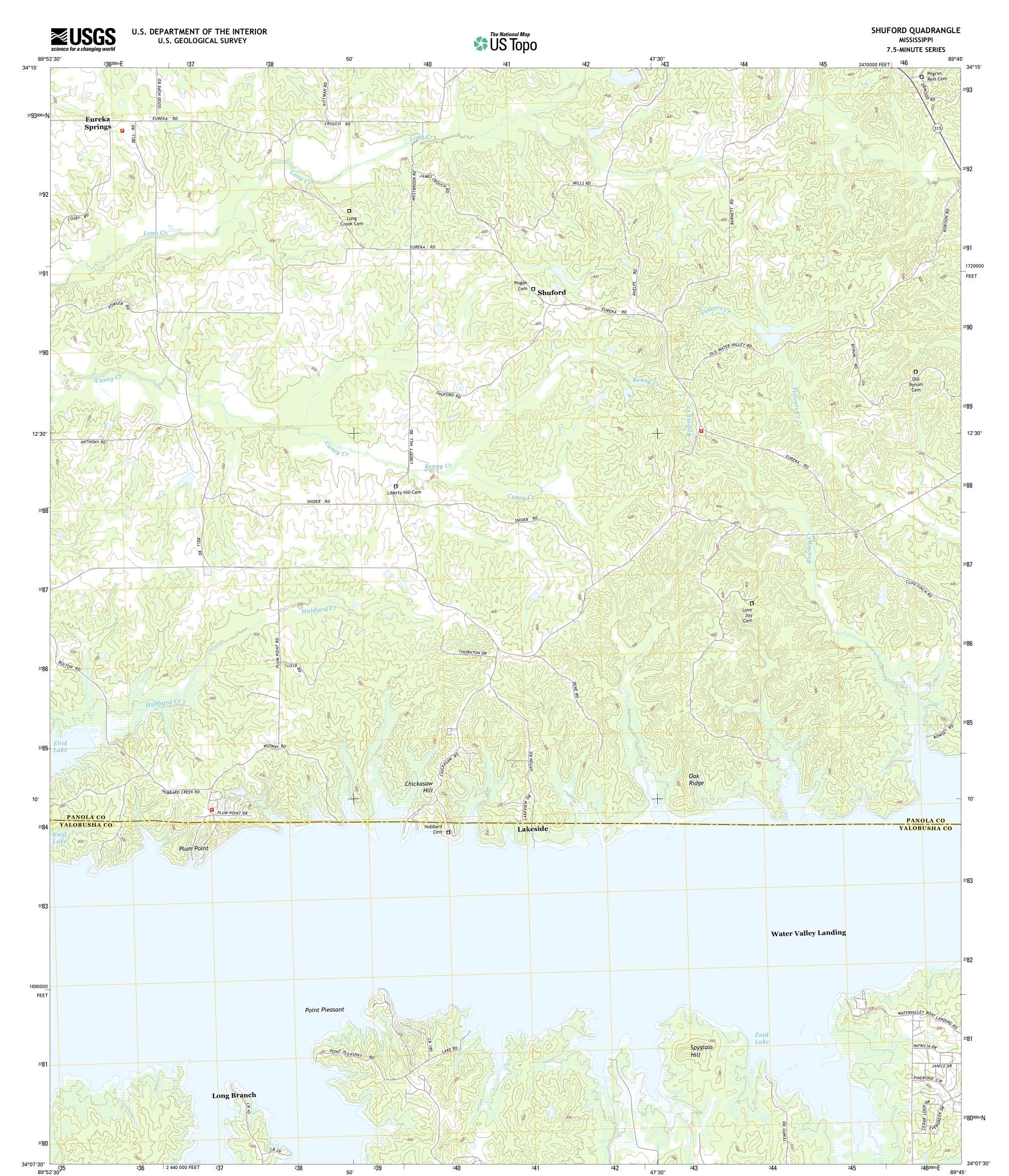
Produced by the United States Geological Survey North American Datum of 1983 (NAD83) World Geodetic System of 1984 (WGS84). Projection and 1 000-meter grid: Universal Transverse Mercator, Zone 16S 10 000-foot ticks: Mississippi Coordinate System of 1983 (west zone)
