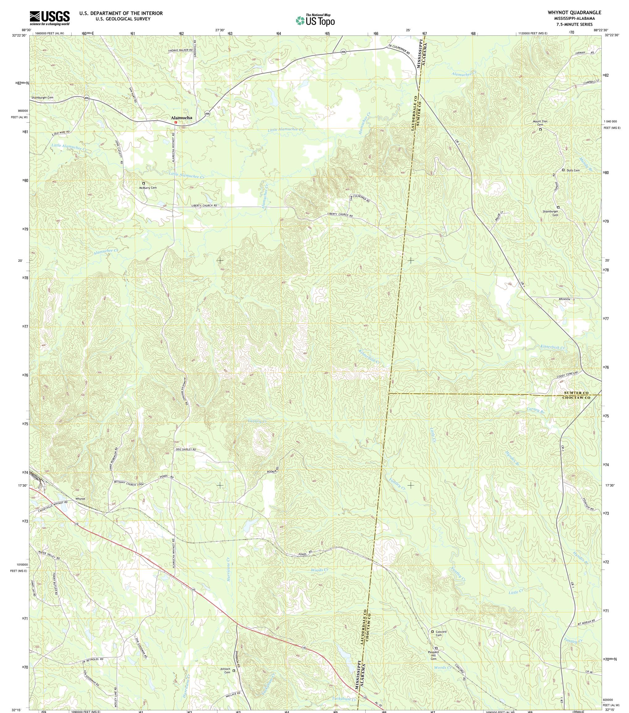
Produced by the United States Geological Survey North American Datum of 1983 (NAD83) World Geodetic System of 1984 (WGS84). Projection and 1 000-meter grid: Universal Transverse Mercator, Zone 16S 10 000-foot ticks: Mississippi Coordinate System of 1983 (east zone), Alabama Coordinate System of 1983 (west zone)
