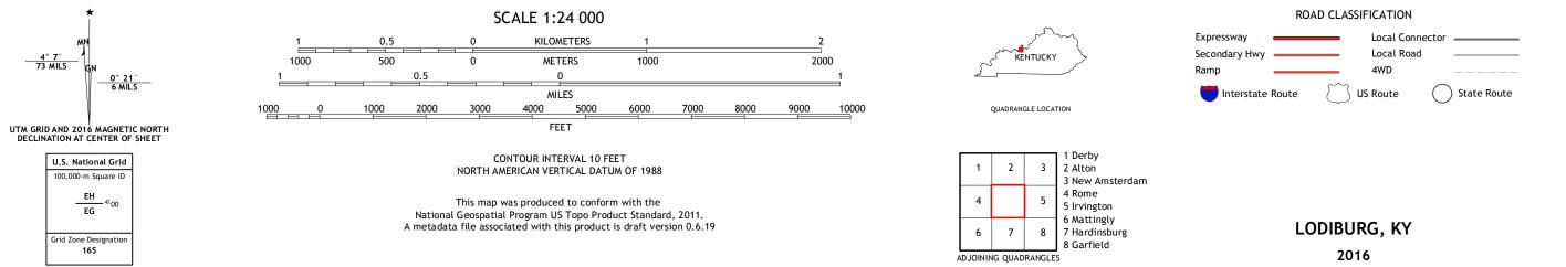
**Produced by the United States Geological Survey** North American Datum of 1983 (NAD83) World Geodetic System of 1984 (WGS84). Projection and 1 000-meter grid: Universal Transverse Mercator, Zone 16S 10 000-foot ticks: Kentucky Coordinate System of 1983 (south Zone) zone)
