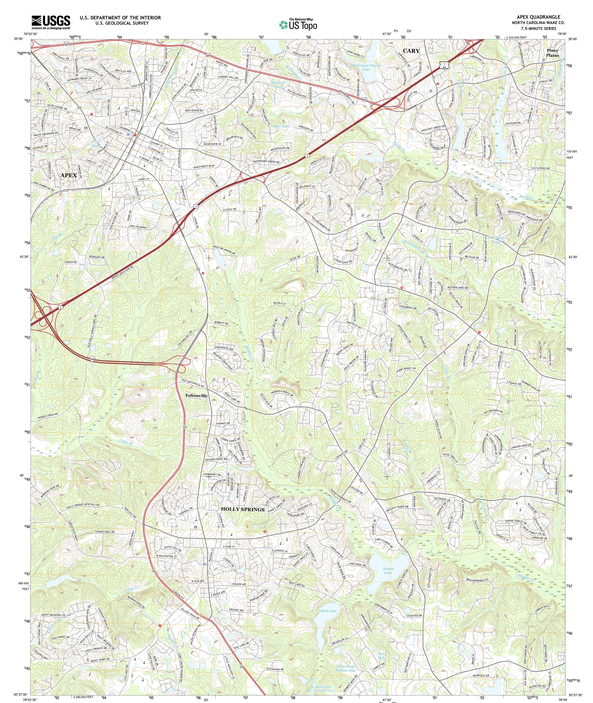
Produced by the United States Geological Survey North American Datum of 1983 (NAD83) World Geodetic System of 1984 (WGS84). Projection and 1 000-meter grid: Universal Transverse Mercator, Zone 17S 10 000-foot ticks: North Carolina Coordinate System of 1983
