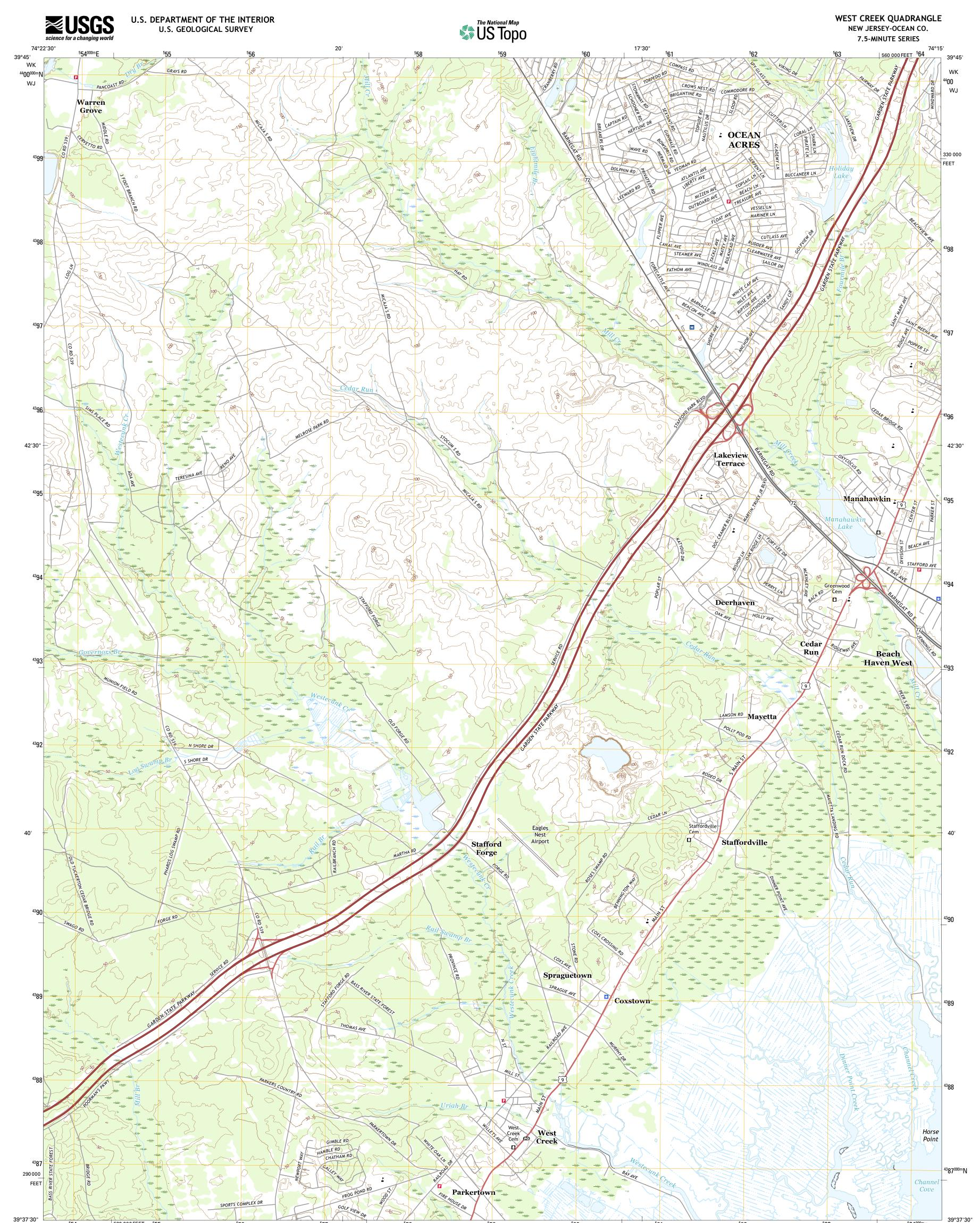
Produced by the United States Geological Survey North American Datum of 1983 (NAD83) World Geodetic System of 1984 (WGS84). Projection and 1 000-meter grid: Universal Transverse Mercator, Zone 18S 10 000-foot ticks: New Jersey Coordinate System of 1983
